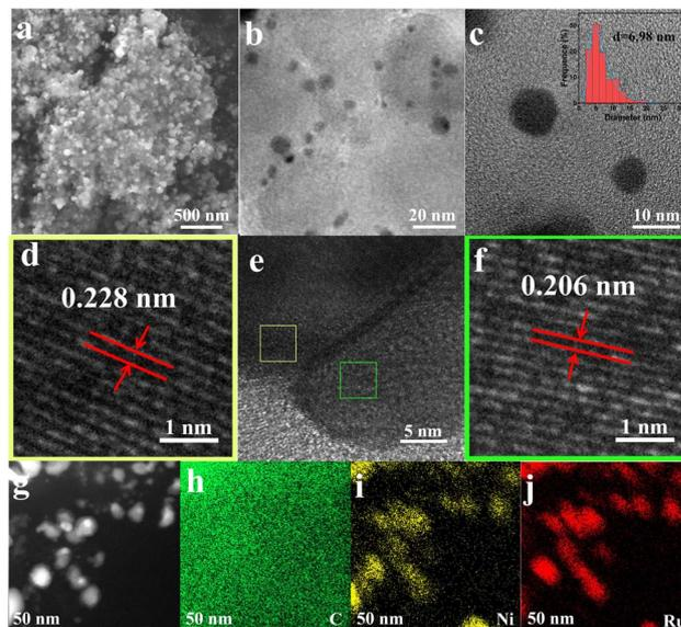
Fig. 2 (a) SEM images of  $\text{Ni}_1\text{Ru}_1/\text{C}$ . (b–e) TEM images of  $\text{Ni}_1\text{Ru}_1/\text{C}$ . (d and f) The enlarged images of the yellow part (d) and green part (f) in (e), respectively. (g–j) STEM/EDS image with elemental mapping images for C, Ni and Ru.
