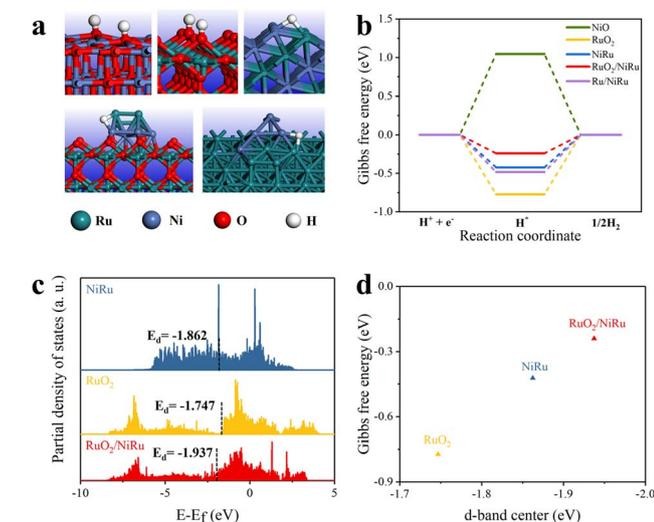
**Fig. 6** (a) Schematic illustration of the adsorption model. (b) Gibbs free energy diagram for hydrogen evolution at equilibrium ( $U = 0$  V) in NiO, RuO<sub>2</sub>, NiRu, and RuO<sub>2</sub>/NiRu interface. (c) PDOS and d-band centers of RuO<sub>2</sub>, NiRu, and RuO<sub>2</sub>/NiRu interface. (d) Gibbs free energy changes of hydrogen adsorption as a function of d-band centers of RuO<sub>2</sub>, NiRu, and RuO<sub>2</sub>/NiRu interface.
