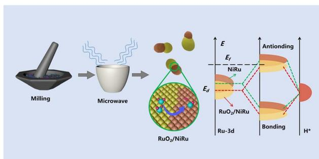
Fig. 1 Schematic illustration of the preparation process of the RuO<sub>2</sub>/NiRu.
