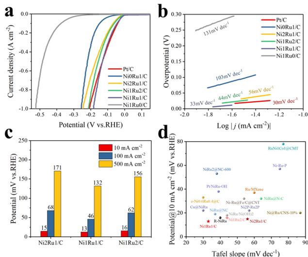
Fig. 3 (a) Polarization curves (with  $iR$  correction) for various electrodes recorded in 1.0 M KOH with a scan rate of  $5 \text{ mV s}^{-1}$ . (b) Tafel plots obtained from the corresponding polarization curves in (a). (c) Comparison of the required overpotentials at 10, 100 and  $500 \text{ mA cm}^{-2}$  for various electrodes. (d) Comparison of NiRu catalysts reported in previous literature based on the potential at  $10 \text{ mA cm}^{-2}$  and Tafel slope.
