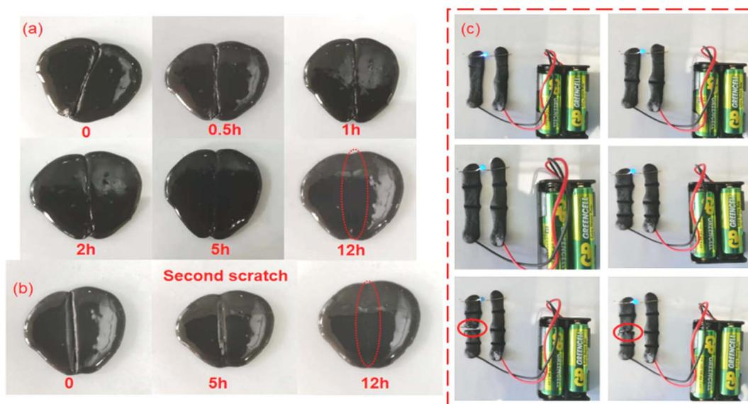
Fig. 7 (a) Self-healing experiment, (b) repeatable self-healing experiment, (c) experiment of self-healing effect on a small bulb, with on and off based on the APC-PVA@ZnCl<sub>2</sub> material.
