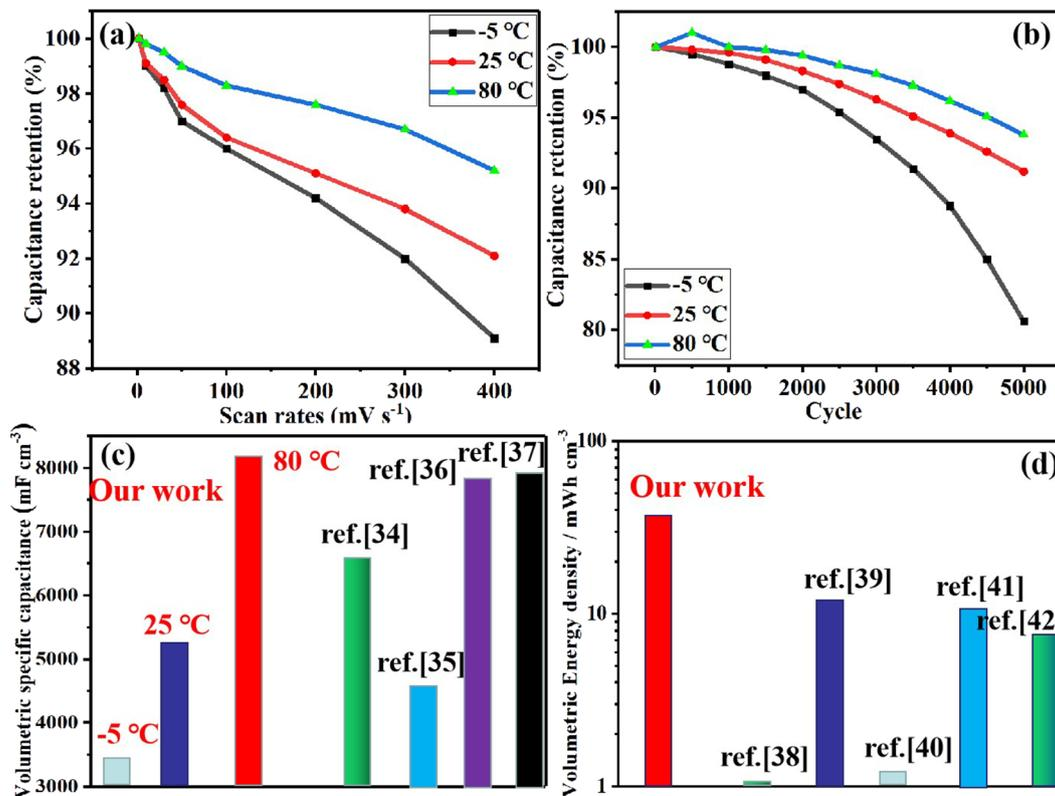
Fig. 4 (a) Capacitance retention of APC-PVA@ZnCl<sub>2</sub> (a) at different temperatures and scan rates. (b) After experiencing 5000 cycles. (c and d) Comparison maps of volumetric specific capacitance and energy density of APC-PVA@ZnCl<sub>2</sub> with reported work.
