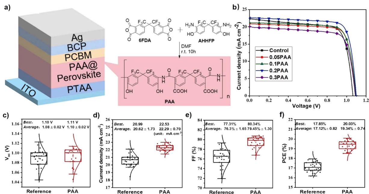
Fig. 1 (a) P-i-n type device architecture and the chemical structure and synthesis procedure of polyamide (PAA), and (b) the  $J$ - $V$  curves for the devices with the additive PAA at a variety of concentrations (0, 0.05, 0.1, 0.2, and 0.3  $\text{mg mL}^{-1}$ ). The statistics of (c)  $V_{\text{OC}}$ ; (d)  $J_{\text{SC}}$ ; (e) FF; and (f) PCE of devices with and without the PAA additive.
