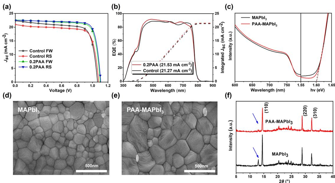
Fig. 2 (a)  $J$ - $V$  curves; (b) EQE spectra and integrated  $J_{SC}$  value versus the wavelength of light for the devices with/without 0.2PAA. (c) Left, UV-Vis absorption spectra; and right, Tauc's plot; top-view SEM images of the perovskite film (d) without and (e) with 0.2PAA passivation; (f) XRD patterns.
