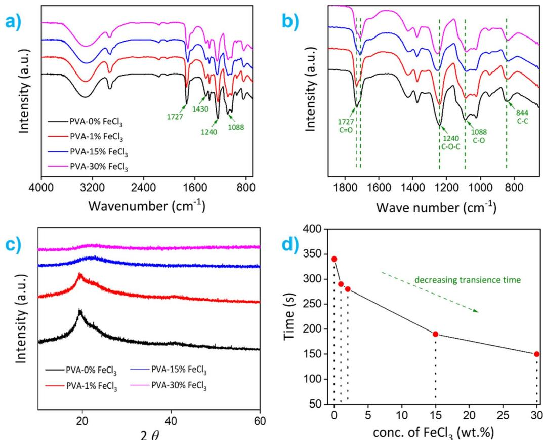
Fig. 2 ATR-FTIR spectra of (a) PVA-FeCl<sub>3</sub> films with additive concentrations of 0, 1, 15, and 30 wt% and (b) enlarged spectra in the wavenumber region from 650 to 1850 cm<sup>-1</sup>. (c) XRD patterns and (d) transience behavior of PVA-FeCl<sub>3</sub> films with different additive concentrations.
