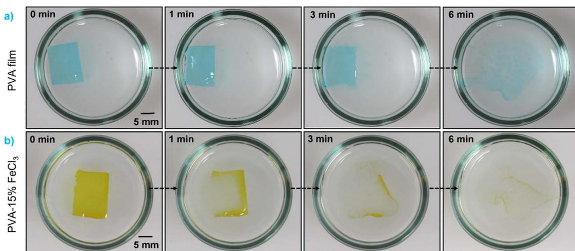
Fig. 1 Digital photographs showing the time-sequential dissolution in distilled water of (a) PVA and (b) PVA-15%  $\text{FeCl}_3$  films with  $M_w$  of 9000–10 000  $\text{g mol}^{-1}$  and 80% degree of hydrolysis.
