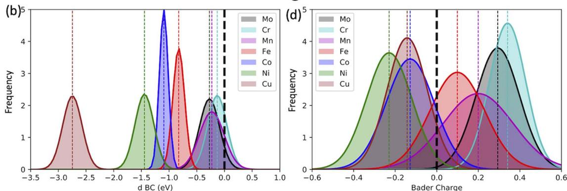
Fig. 5 Normal distribution of the *d* BC (a and b) and Bader charges (c and d) of the adsorbing elements of the 556 randomly created microstructures. Here, elements placed on the subsurface and surface of the microstructures are differentiated. Surface elements are accounted for in (a) and (b), while subsurface atoms are considered in (b) and (d). Subsurface atoms are the referent elements on the second layer of the slab from top to bottom.
