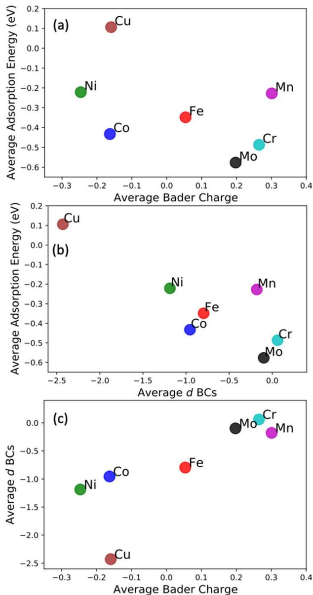
Fig. 7 Average  $N_2$  adsorption energies on the adsorbing atoms Mo, Cr, Mn, Fe, Co, Ni, Cu vs. their averaged Bader charges (a), averaged d BCs (b). (c) Represents the relations between averaged d BCs and averaged Bader charge.
