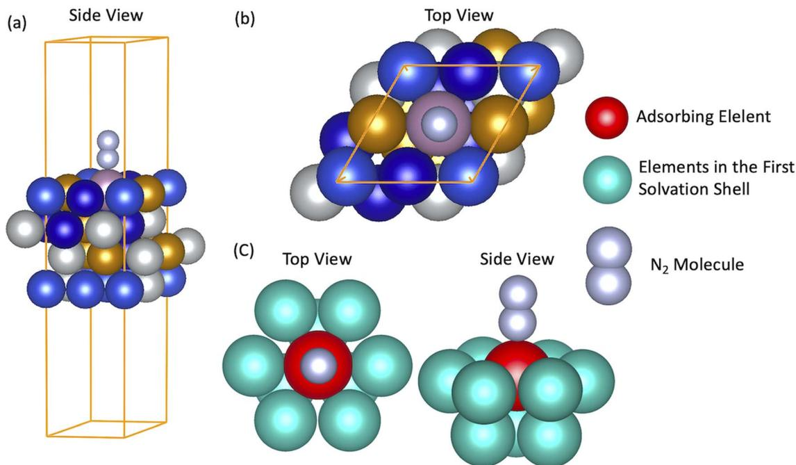
**Fig. 1** Side and top views of one example of microstructure formed with Mo–Fe–Co–Ni–Cu, (a) and (b). The concept of the first solvation shell (here defined as the closest atoms around the element where N<sub>2</sub> is adsorbing) clarifies the bond formation mechanism of N<sub>2</sub> on the HEAs surfaces. Here, light blue elements are in the first solvation shell of the adsorbing atom (red color) (c).
