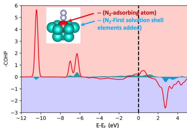
Fig. 4 Projected crystal orbital Hamiltonian population (*-pCOHP*) analysis for the bonds between N<sub>2</sub> and the adsorbing atoms and between N<sub>2</sub> and the first solvation shell. The used model is shown in Fig. 2 (the case of 16 atoms). The red represents the summed-up interactions between N<sub>2</sub> and the adsorbing element while light blue represents summed pairs of elements from the first solvation shell and N<sub>2</sub>.
