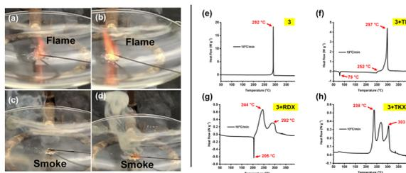
Fig. 8 (a–d) Hot needle tests of compounds 2–5. (e) DSC analysis of 3 at heating rate 10 °C min<sup>-1</sup> (f) DSC analysis of 3:TNT (1 : 1) (g) DSC analysis of 3:RDX (1 : 1) (h) DSC analysis of 3:TKX-50 (1 : 1).
