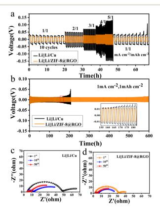
Fig. 3 Electrochemical performance evaluation of Lilli half cells. Comparison of (a) the rate performance and (b) the cycling stability of Cu foil and ZIF-8@RGO in symmetric cells. Insets: magnified profiles during different periods. EIS spectra of (c) bare Cu and (d) ZIF-8@RGO for different cycles at 1 mA cm<sup>-2</sup> for 1 mA h cm<sup>-2</sup>.
