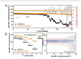
Fig. 5 Electrochemical performance evaluation in full cells. (a) Cycling performances. (b) Rate capabilities of full cells with two types of anodes at 0.5C coupled with LiFePO $_4$  cathode. (c) The corresponding charge—discharge profiles at different rates with Li/ZIF-8@RGO as anode.
