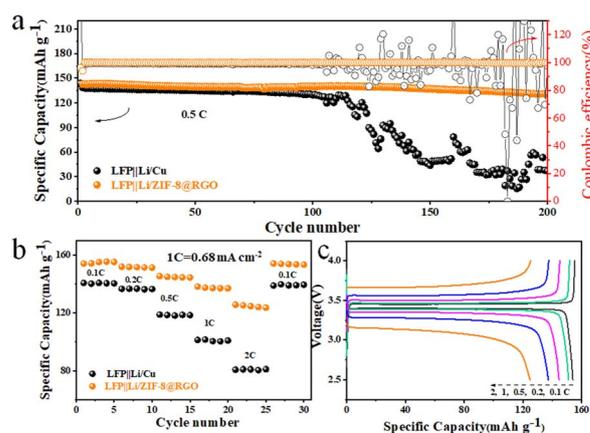
Fig. 5 Electrochemical performance evaluation in full cells. (a) Cycling performances. (b) Rate capabilities of full cells with two types of anodes at 0.5C coupled with LiFePO<sub>4</sub> cathode. (c) The corresponding charge-discharge profiles at different rates with Li/ZIF-8@RGO as anode.
