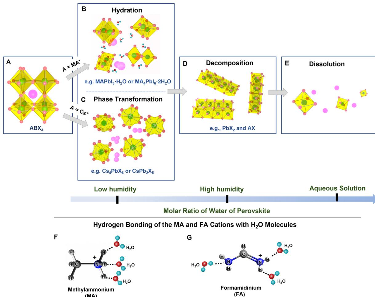
Fig. 1 (A–E) Schematic representations of the interactions between water molecules and halide PeNCs (modified with permission from ref. 26). (F and G) Schematic representations of the formation of the hydrogen bonding of methylammonium (F) and formamidineum (G) cations with water molecules.
