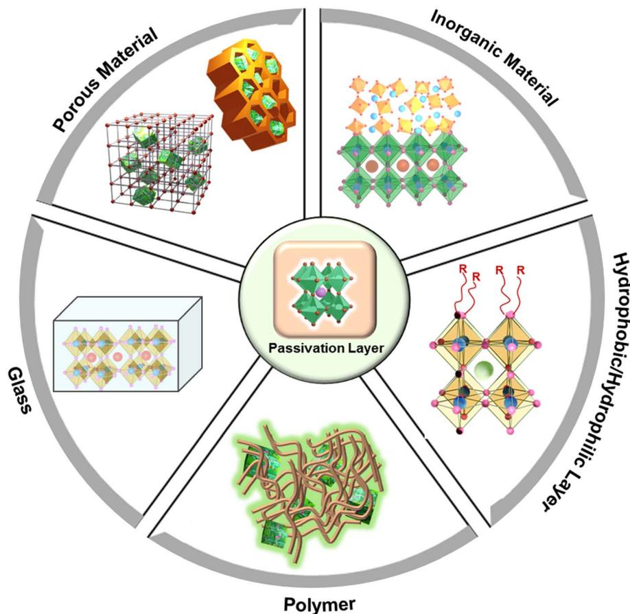
Fig. 4 A schematic representation of the various methods for surface passivation of PeNCs.
