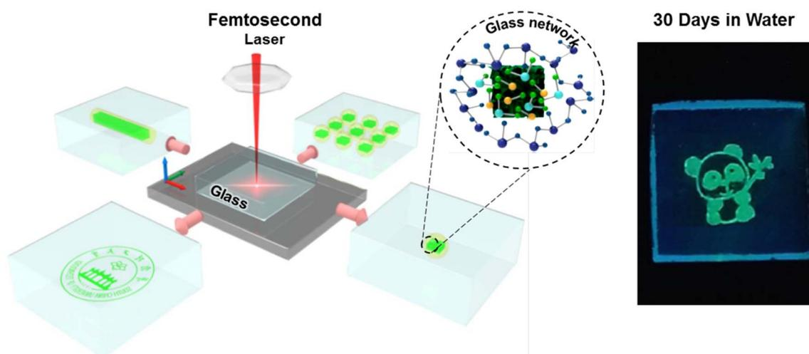
Fig. 9 Scheme of the 3D perovskite patterns generated inside the glass matrix by using femtosecond laser irradiation and the digital image of CsPbBr<sub>3</sub> patterns after being stored in water for 30 days (modified with permission from ref. 41).
