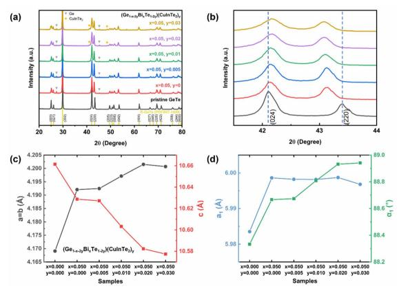
Fig. 1 (a) XRD patterns of  $(Ge_{1-x-2y}Bi_xTe_{1-2y})(CuInTe_2)_y$  (x=0 and 0.05; y=0.005, 0.01, 0.02, and 0.03) samples. (b) Enlarged diffraction peaks of (024) and (220) in (a). (c) Experimental lattice parameters of  $(Ge_{1-x-2y}Bi_xTe_{1-2y})(CuInTe_2)_y$ . (d) The refined lattice parameter and interaxial angle based on a pseudo cubic unit cell.
