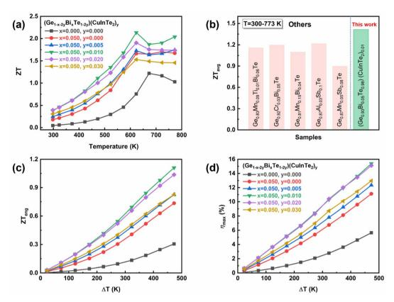
Fig. 7 (a) Temperature-dependent ZT of  $(Ge_{1-x-2y}Bi_xTe_{1-2y})(CuInTe_2)_y$  samples and (b) the average ZT value with other reported GeTe compounds. (c) The  $ZT_{eng}$  values and (d)  $\eta_{max}$  values of  $(Ge_{1-x-2y}Bi_xTe_{1-2y})(CuInTe_2)_y$  samples.
