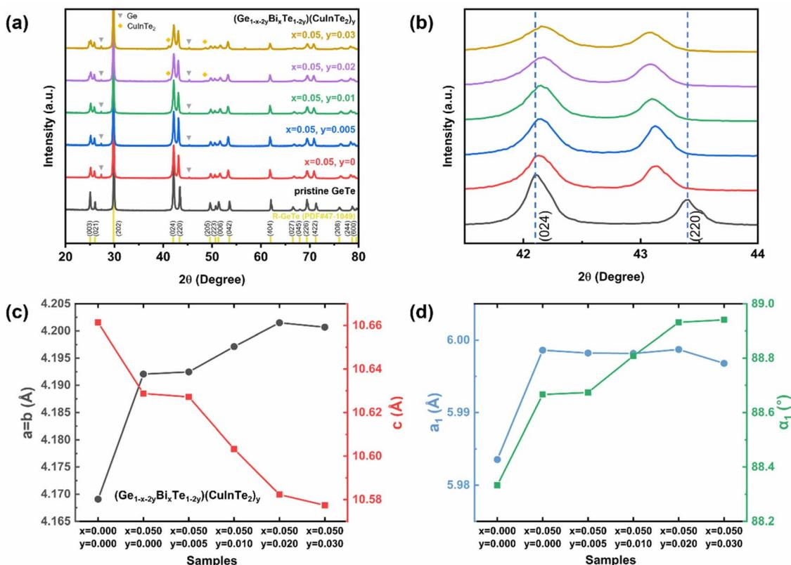
Fig. 1 (a) XRD patterns of  $(\text{Ge}_{1-x-2y}\text{Bi}_x\text{Te}_{1-2y})(\text{CuInTe}_2)_y$  ( $x = 0$  and  $0.05; y = 0.005, 0.01, 0.02, \text{ and } 0.03$ ) samples. (b) Enlarged diffraction peaks of (024) and (220) in (a). (c) Experimental lattice parameters of  $(\text{Ge}_{1-x-2y}\text{Bi}_x\text{Te}_{1-2y})(\text{CuInTe}_2)_y$ . (d) The refined lattice parameter and interaxial angle based on a pseudo cubic unit cell.
