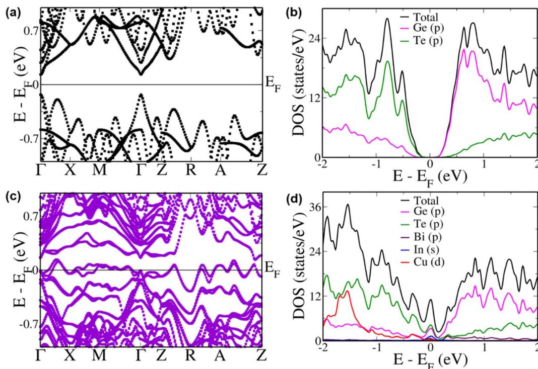
Fig. 4 Electronic structure and pDOS of cubic (a and b)  $\text{Ge}_{16}\text{Te}_{16}$ ; (c and d)  $\text{Ge}_{13}\text{BiInCuTe}_{16}$ .
