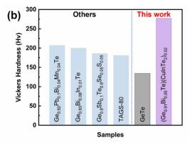
Fig. 8 (a) Vickers hardness values of  $(Ge_{1-x-2\nu}Bi_xTe_{1-2\nu})(CuInTe_2)_v$  samples and (b) compared with those of other reported GeTe samples.
