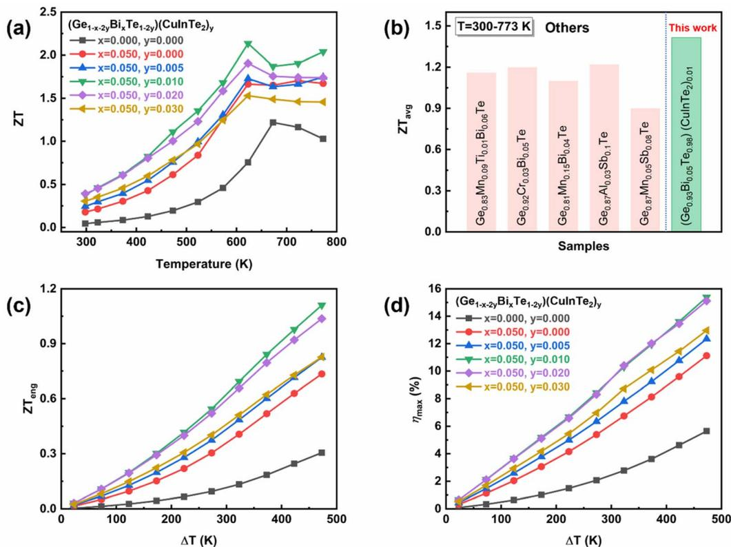
Fig. 7 (a) Temperature-dependent  $ZT$  of  $(\text{Ge}_{1-x-2y}\text{Bi}_x\text{Te}_{1-2y})(\text{CuInTe}_2)_y$  samples and (b) the average  $ZT$  value with other reported GeTe compounds. (c) The  $ZT_{\text{eng}}$  values and (d)  $\eta_{\text{max}}$  values of  $(\text{Ge}_{1-x-2y}\text{Bi}_x\text{Te}_{1-2y})(\text{CuInTe}_2)_y$  samples.
