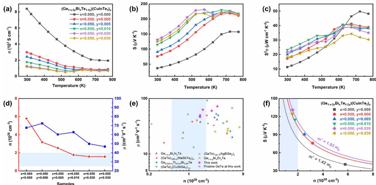
Fig. 3 Temperature-dependent (a) electrical conductivity, (b) Seebeck coefficient, and (c) power factor of  $(\text{Ge}_{1-x-2y}\text{Bi}_x\text{Te}_{1-2y})(\text{CuInTe}_2)_y$  samples. (d) Composition-dependent Hall carrier concentration and Hall mobility at room temperature. Carrier concentration-dependent (e) Hall mobility in comparison with other reported data and (f) the Seebeck coefficient at room temperature.
