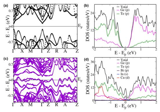
Fig. 4 Electronic structure and pDOS of cubic (a and b) Ge<sub>16</sub>Te<sub>16</sub>; (c and d) Ge<sub>13</sub>BilnCuTe<sub>16</sub>.
