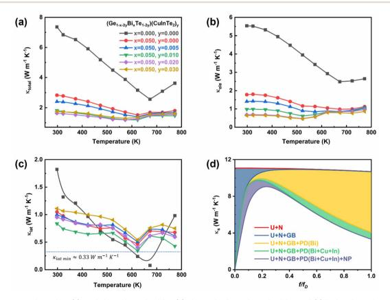
Fig. 6 Temperature-dependent (a) total thermal conductivity, (b) electronic thermal conductivity, and (c) lattice thermal conductivity of  $(Ge_{1-x-2y}Bi_xTe_{1-2y})(CuInTe_2)_y$  samples. (d) Calculated spectral lattice thermal conductivity as a function of phonon frequency (f) based on various phonon scattering processes including the normal process (N), the Umklapp process (U), grain boundaries (GB), point defects (PD), and nanoprecipitate (NP) at 300 K.
