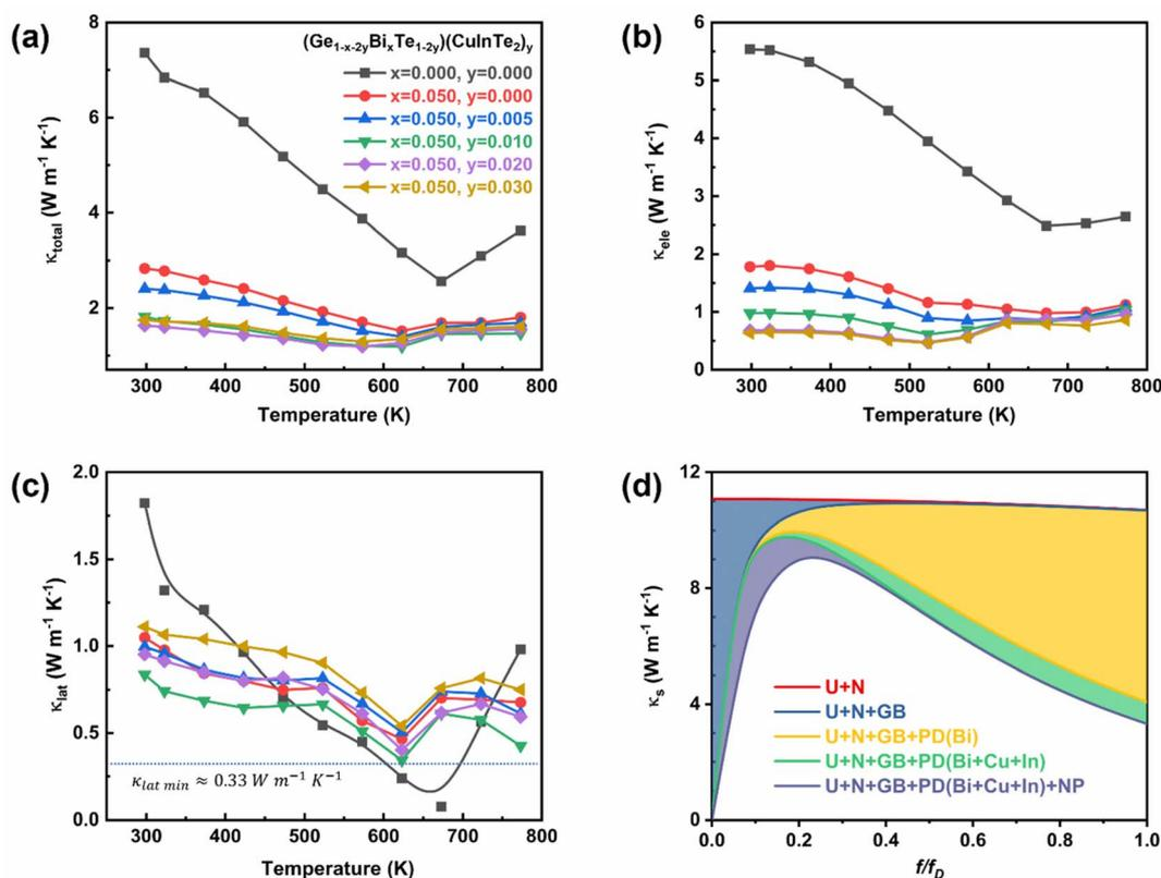
Fig. 6 Temperature-dependent (a) total thermal conductivity, (b) electronic thermal conductivity, and (c) lattice thermal conductivity of  $(\text{Ge}_{1-x-2y}\text{Bi}_x\text{Te}_{1-2y})(\text{CuInTe}_2)_y$  samples. (d) Calculated spectral lattice thermal conductivity as a function of phonon frequency ( $f$ ) based on various phonon scattering processes including the normal process (N), the Umklapp process (U), grain boundaries (GB), point defects (PD), and nanoprecipitate (NP) at 300 K.
