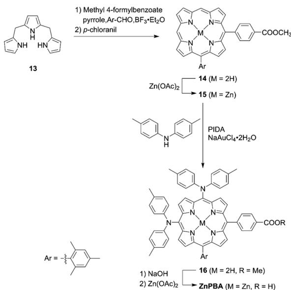
Scheme 3 Synthesis of ZnPBAT. PIDA = phenyliodine(III) diacetate.
