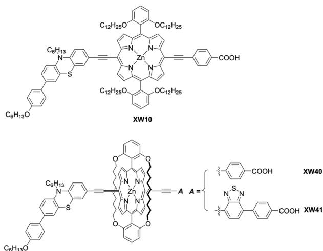
Fig. 15 Chemical structures of **XW40**, **XW41**, and **XW10**.
