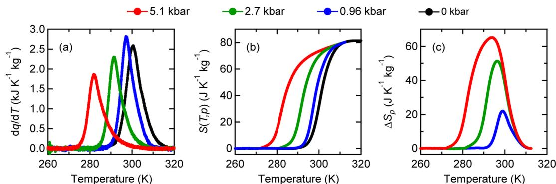
**Fig. 2** (a) Heat flow curves divided by the cooling rate  $dq/dT$ , (b) corresponding entropy as a function of temperature, and (c) isothermal entropy changes of  $\text{NdCu}_3\text{Fe}_4\text{O}_{12}$  under various applied pressures.
