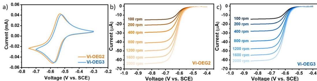
Fig. 2 (a) Cyclic voltammograms of Vi-OEG2 and Vi-OEG3. Condition: 5 mM viologens in 0.5 M NaBr aqueous electrolyte at a scan rate of  $50 \text{ mV s}^{-1}$ . Linear sweep voltammograms of (b) Vi-OEG2 and (c) Vi-OEG3. Condition: 1 mM viologens in 0.5 M NaCl aqueous electrolyte at a scan rate of  $5 \text{ mV s}^{-1}$ .
