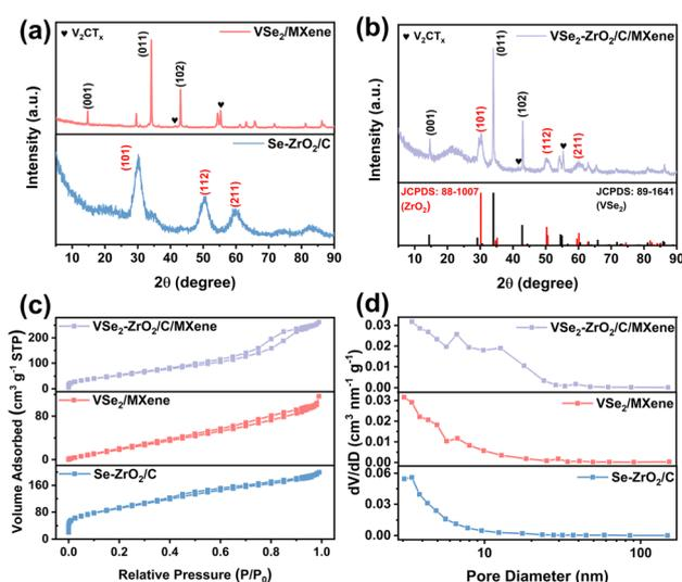
Fig. 2 XRD patterns of (a)  $VSe_2/MXene$  and  $Se-ZrO_2/C$ , (b)  $VSe_2-ZrO_2/C/MXene$ . (c) Nitrogen adsorption–desorption isotherms and (d) pore size distributions of  $VSe_2-ZrO_2/C/MXene$ ,  $VSe_2/MXene$  and  $Se-ZrO_2/C$ .
