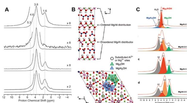
Fig. 5 (A) Solid-state  $^1\text{H}$  NMR spectra of Mg/Al-2-LDH. (B) Schematic illustration of Mg/Al-2-LDH. (C) Quantitative fitting of the  $^1\text{H}$  echo-MAS NMR spectra of LDH.<sup>81</sup> Copyright © 2011 American Chemical Society.
