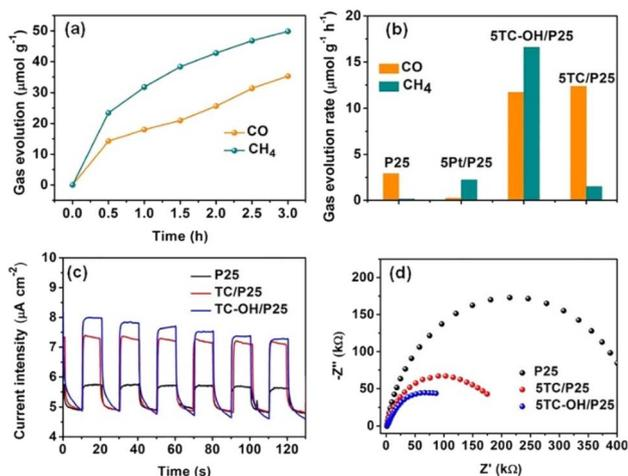
Fig. 10 (a) Gas evolution (CO and CH<sub>4</sub>) over 5TC-OH/P25 as a function of irradiation time under a 300 W Xe lamp. (b) Evolution rates of CO and CH<sub>4</sub> over P25, 5Pt/P25, 5TC/P25, and 5TC-OH/P25 under irradiation of a 300 W Xe lamp. (c) Transient photocurrent responses and (d) EIS Nyquist plots of P25, 5TC/P25, and 5TC-OH/P25. Reproduced with permission from ref. 131, Copyright 2018 European Chemical Societies Publishing.
