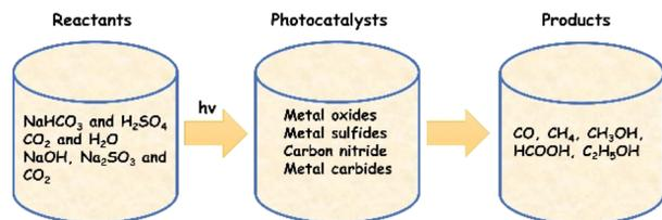
Fig. 9 Schematic representation of photocatalytic CO<sub>2</sub> conversion highlighting frequently used reactants, photocatalysts and possible products that can be formed.
