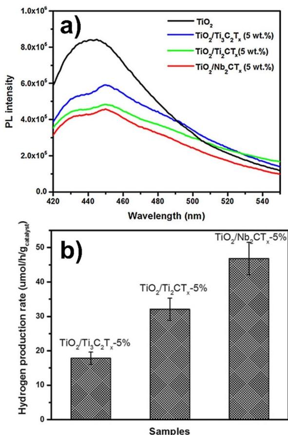
Fig. 6 (a) Photoluminescence spectra of pure  $\text{TiO}_2$  along with those of the materials with different 5 wt% metal carbide cocatalysts. The excitation wavelength was 400 nm. (b) Photocatalytic hydrogen production rates obtained for different metal carbide cocatalysts. Reproduced with permission from ref. 97, Copyright 2016 European Chemical Societies Publishing.
