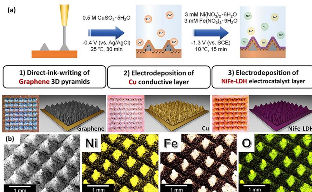
**Fig. 7** (a) Schematic illustration of the fabrication of 3D-printed pyramid electrodes for OER in three successive steps. (1) Direct-ink-writing of graphene 3D pyramid array, electrodeposition of (2) Cu conductive layer and (3) NiFe-layered double hydroxide (LDH) electrocatalyst layers. (b) Energy dispersive spectrometry (EDS) mapping images of NiFe-LDH pyramid electrode: Ni (yellow), Fe (apricot), and O (green) (reproduced from ref. 113 with permission).
