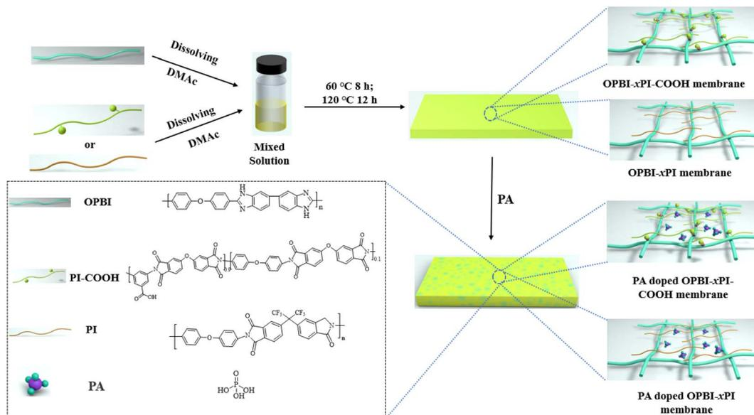
Scheme 2 Preparation of OPBI-xPI-COOH and OPBI-xPI membranes.
