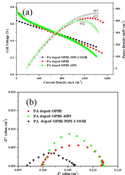
Fig. 8 (a) Polarization and power density profiles of PA-doped membranes for HT-PEMFCs at 160 °C, and (b) *in situ* impedance spectra of the MEAs with different PA-doped membranes at a cell voltage of 0.7 V and 160 °C.
