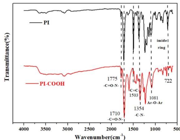
Fig. 2 FT-IR spectrum of PI and PI-COOH.
