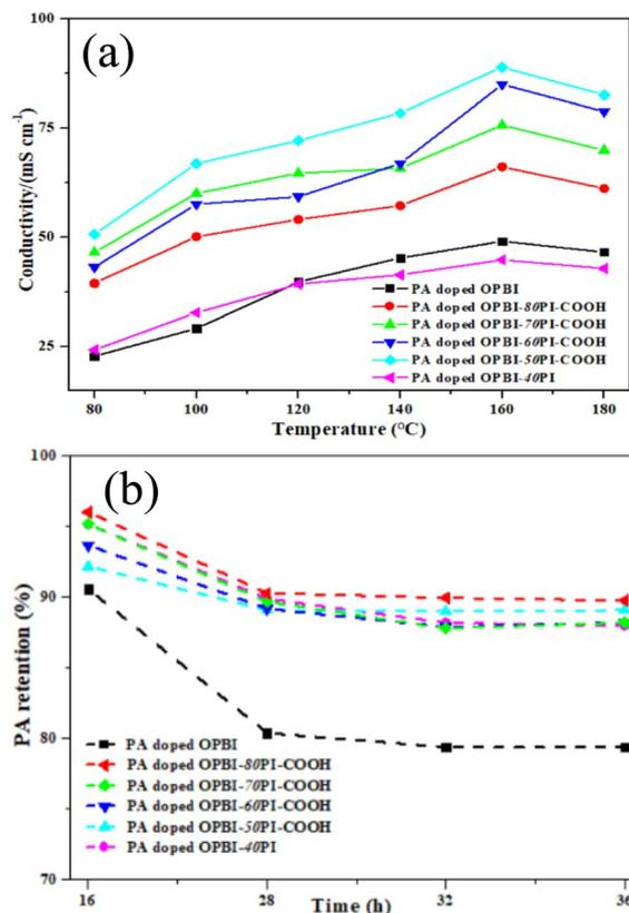
Fig. 5 (a) Proton conductivity plots of PA-doped OPBI, OPBI-*x*PI-COOH, and OPBI-40PI membranes at different temperatures without humidification; (b) PA retention of PA-doped OPBI, OPBI-*x*PI-COOH, and OPBI-40PI membranes at  $80\text{ °C}$  with 0% relative humidity.
