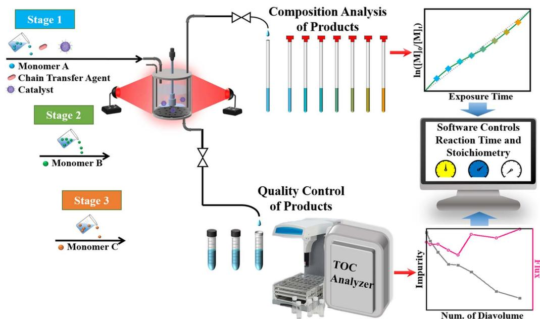
Scheme 2 Schematic diagram of the SCBMR system designed for the cascade synthesis of block copolymers.
