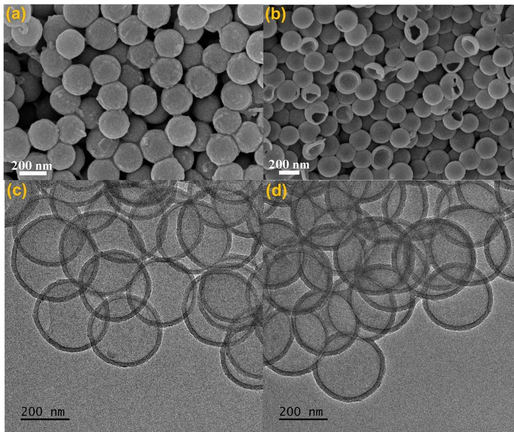
Fig. 1 Morphological observation: FESEM and TEM images of (a) SiO<sub>2</sub>@H-PPrIB-2, (b and c) H-PPrIB-2 and (d) H-PPrIB-M microspheres.
