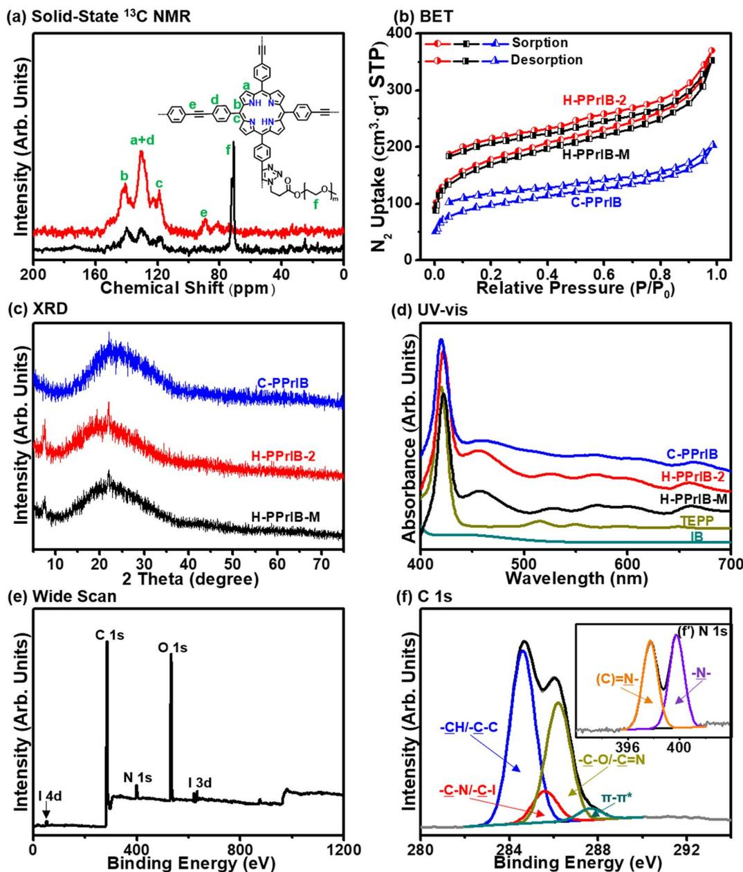
Fig. 2 Structural characterization: (a) solid-state  $^{13}\text{C}$  NMR spectra of H-PPriB-M and H-PPriB-2 MSs; (b)  $\text{N}_2$  isotherms of H-PPriB-M, H-PPriB-2 MSs and C-PPriB CMPs at 77 K with respective BET surface areas estimated to be 600.5, 630.8 and 346.9  $\text{m}^2 \text{g}^{-1}$ , respectively; (c) XRD patterns and (d) UV-visible spectra of H-PPriB-M, H-PPriB-2 MSs and C-PPriB CMPs; (e) XPS wide scan, (f) C 1s and (f') N 1s core-level spectra of H-PPriB-M MSs.
