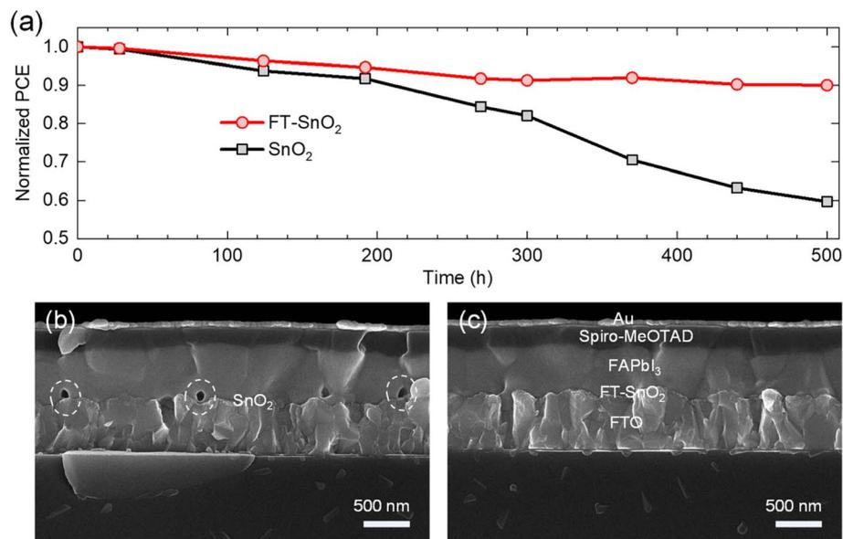
Fig. 5 (a) Comparison of normalized PCE of PSCs based on bare SnO<sub>2</sub> and FT-SnO<sub>2</sub>. The devices were stored in the dark at room temperature and under relative humidity of 25 ± 10% for 500 h. Cross-sectional SEM images of the 500 h-aged PSCs based on (b) bare SnO<sub>2</sub> and (c) FT-SnO<sub>2</sub>.
