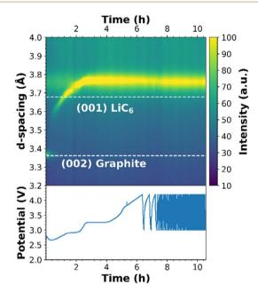
Fig. 13 Densiometric view of diffraction patterns during *operando*-SXRD of a NMC622 vs. graphite pouch cell (top) and the corresponding electrochemical behavior (bottom).
