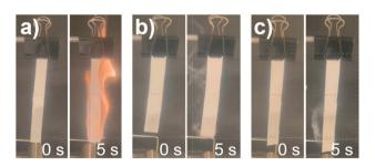
Fig. 2 An overview of the flammability experiment. Figure (a) represents LP40, figure (b) represents 1.5 M LiFSI in TEP/BTFE and figure (c) represents 1.5 M LiFSI in TEP/TTE.
