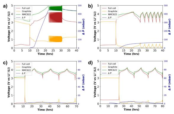
Fig. 11 Pressure evolution in 3-electrode cells with NMC622 vs. graphite (Li-metal reference). (a) 1.0 M LiFSI in TEP, (b) 3.0 M LiFSI in TEP, (c) 1.5 M LiFSI in TEP/BTFE and (d) 1.5 M LiFSI in TEP/TTE.
