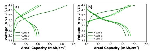
Fig. 12 Discharge capacities of 3-electrode cells with NMC622 vs. graphite (Li-metal reference), using (a) BTFE-based electrolyte and (b) TTE-based electrolyte.
