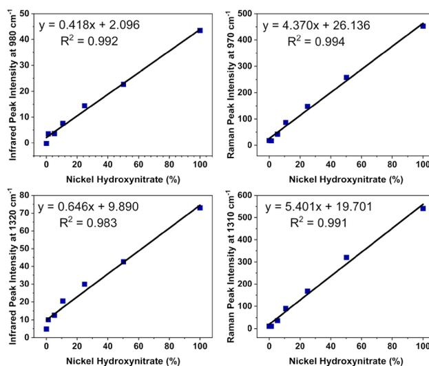
Fig. 8 Calibration plots showing the linear relationship between the background-corrected intensity observed of the  $C_{2v}$  nitrate infrared band at 980  $\text{cm}^{-1}$  and 1320  $\text{cm}^{-1}$  as well as Raman band at 970  $\text{cm}^{-1}$  1310  $\text{cm}^{-1}$  with the weight percentage (wt%) proportion of nickel hydroxynitrate present.
