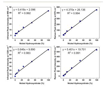
Fig. 8 Calibration plots showing the linear relationship between the background-corrected intensity observed of the  $C_{2v}$  nitrate infrared band at 980 cm<sup>-1</sup> and 1320 cm<sup>-1</sup> as well as Raman band at 970 cm<sup>-1</sup> 1310 cm<sup>-1</sup> with the weight percentage (wt%) proportion of nickel hydroxynitrate present.
