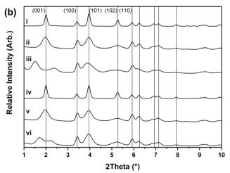
Fig. 4 Powder X-ray diffraction patterns collected with (a) Cu  $\rm K_{z1}$  ( $\lambda$  = 1.5406 Å) and (b) synchrotron ( $\lambda$  = 0.161669 Å) radiation of the i–vi nickel hydroxide materials. The *hkl* assignments given are of nickel hydroxide (ICDD PDF 14-117).
