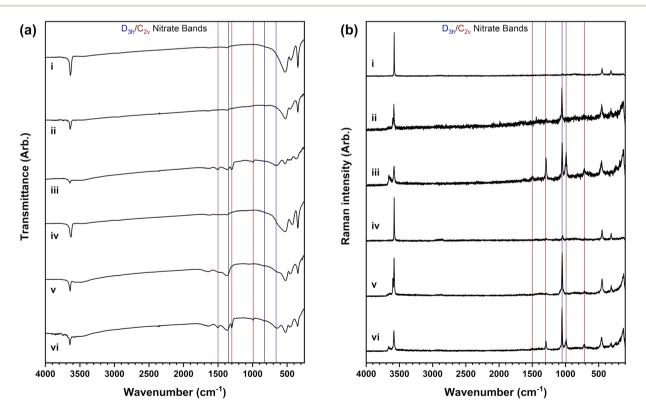
Fig. 6 (a) Infrared spectra and (b) Raman spectra of the i-vi nickel hydroxide materials. The vertical lines indicate nitrate bands, with the  $D_{3h}$ symmetry (blue lines) indicating loosely held nitrate between the layers in alpha-phase layered hydroxides as well as the cation coordinated  $C_{2\nu}$ symmetry (red lines) associated with layered hydroxynitrates.
