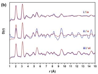
Fig. 5 X-ray pair distribution function data collected with synchrotron radiation ( $\lambda = 0.161669 \text{ Å}$ ) of the i–vi nickel hydroxide materials. (a) A comparison of the observed atomic pair distances to the interlayer and intralayer distances expected of beta-phase nickel hydroxide and (b) an overlay comparison of the individual material types
