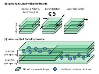
Fig. 2 (a) Diagram of stacking fault disorder in adjacent beta-phase nickel hydroxide layers (left) including rotation about the c-axis (centre) and translation in the ab-plane (right).  $^{34}$  (b) Diagram of the phase interstratification that occurs within a single crystal of nickel hydroxide highlighting regions of beta-phase as well as alpha-phase nickel hydroxide with intercalating species.  $^{40}$
