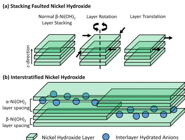
Fig. 2 (a) Diagram of stacking fault disorder in adjacent beta-phase nickel hydroxide layers (left) including rotation about the  $c$ -axis (centre) and translation in the  $ab$ -plane (right).<sup>34</sup> (b) Diagram of the phase interstratification that occurs within a single crystal of nickel hydroxide highlighting regions of beta-phase as well as alpha-phase nickel hydroxide with intercalating species.<sup>40</sup>
