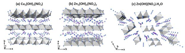
Fig. 3 The crystal structures of the layered hydroxynitrate phases (a)  $Cu_2(OH)_3(NO_3)$  (gerhardtite) where x = 0.5, (b)  $Zn_3(OH)_4(NO_3)_2$  where x = 0.50.67, and (c)  $Zn(OH)(NO_3) \cdot H_2O$  where x = 1.0. Metal(II) cations form coordination octahedra (grey) with the oxygen (blue spheres) of the hydroxide groups or the nitrate groups (nitrogen are purple spheres).
