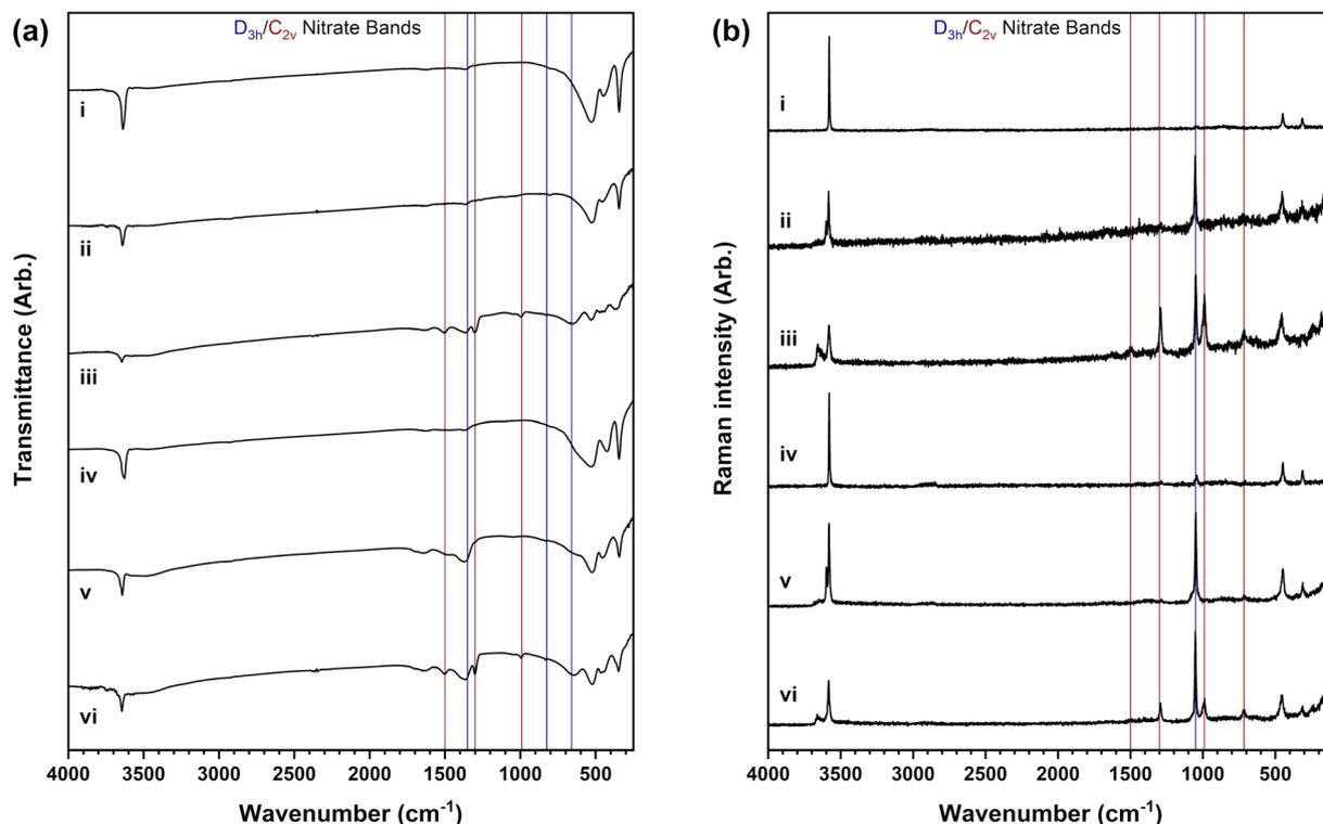
Fig. 6 (a) Infrared spectra and (b) Raman spectra of the i–vi nickel hydroxide materials. The vertical lines indicate nitrate bands, with the  $D_{3h}$  symmetry (blue lines) indicating loosely held nitrate between the layers in alpha-phase layered hydroxides as well as the cation coordinated  $C_{2v}$  symmetry (red lines) associated with layered hydroxynitrates.
