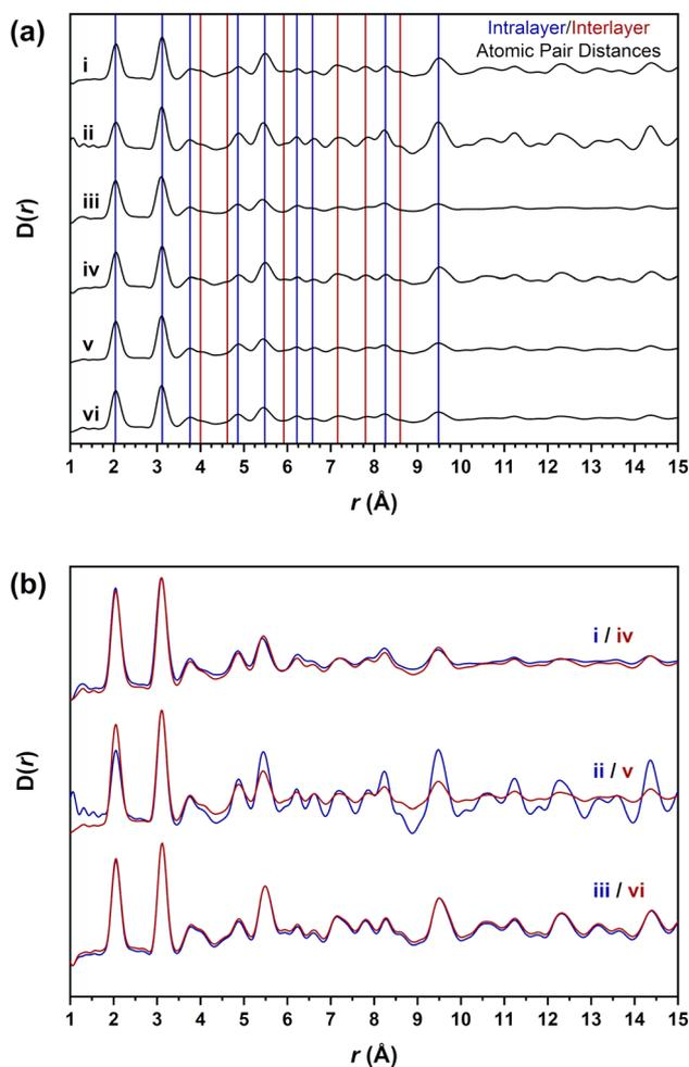
Fig. 5 X-ray pair distribution function data collected with synchrotron radiation ( $\lambda = 0.161669$  Å) of the  $i$ - $vi$  nickel hydroxide materials. (a) A comparison of the observed atomic pair distances to the interlayer and intralayer distances expected of beta-phase nickel hydroxide and (b) an overlay comparison of the individual material types.
