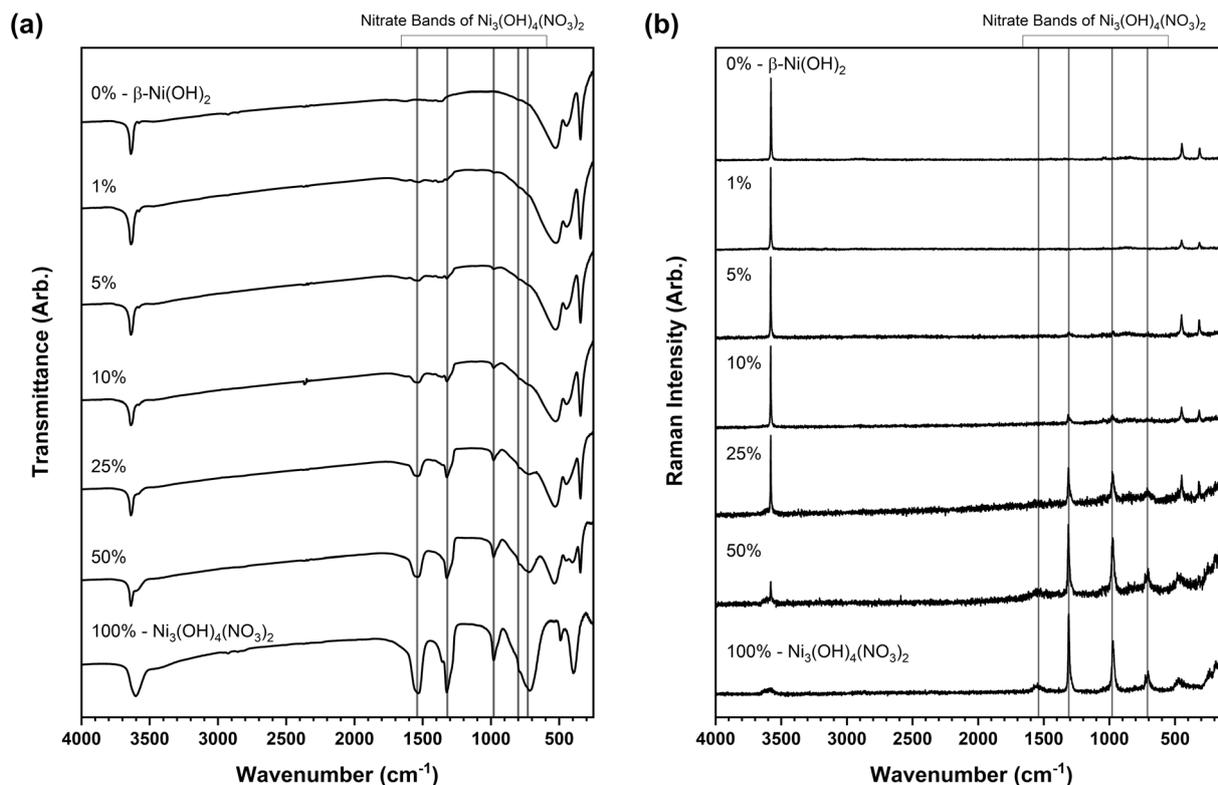
Fig. 7 (a) Infrared absorption spectra as CsI disks and (b) Raman spectra collected for the standard mixtures formed between  $\beta$ -Ni(OH)<sub>2</sub> and the layered hydroxynitrate Ni<sub>3</sub>(OH)<sub>4</sub>(NO<sub>3</sub>)<sub>2</sub> at 0, 1, 5, 10, 25, 50 and 100 wt% intervals.
