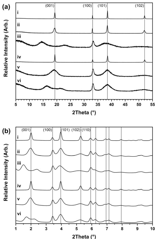
Fig. 4 Powder X-ray diffraction patterns collected with (a) Cu  $K_{\alpha 1}$  ( $\lambda = 1.5406$  Å) and (b) synchrotron ( $\lambda = 0.161669$  Å) radiation of the i–vi nickel hydroxide materials. The  $hkl$  assignments given are of nickel hydroxide (ICDD PDF 14-117).
