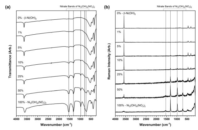
Fig. 7 (a) Infrared absorption spectra as CsI disks and (b) Raman spectra collected for the standard mixtures formed between β-Ni(OH)<sub>2</sub> and the layered hydroxynitrate Ni<sub>3</sub>(OH)<sub>4</sub>(NO<sub>3</sub>)<sub>2</sub> at 0, 1, 5, 10, 25, 50 and 100 wt% intervals.
