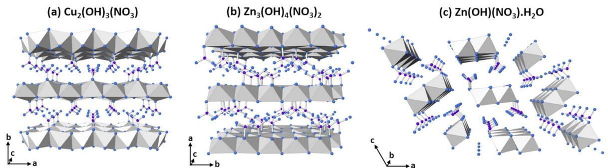
Fig. 3 The crystal structures of the layered hydroxynitrate phases (a)  $\text{Cu}_2(\text{OH})_3(\text{NO}_3)$  (gerhardtite) where  $x = 0.5$ , (b)  $\text{Zn}_3(\text{OH})_4(\text{NO}_3)_2$  where  $x = 0.67$ , and (c)  $\text{Zn}(\text{OH})(\text{NO}_3) \cdot \text{H}_2\text{O}$  where  $x = 1.0$ . Metal(II) cations form coordination octahedra (grey) with the oxygen (blue spheres) of the hydroxide groups or the nitrate groups (nitrogen are purple spheres).
