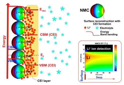
Fig. 1 Schematics of energy band bending with cathode-electrolyte interphase (CEI) layer formation and the visualization of the Li<sup>+</sup> by SIMS positive ion detection mode.
