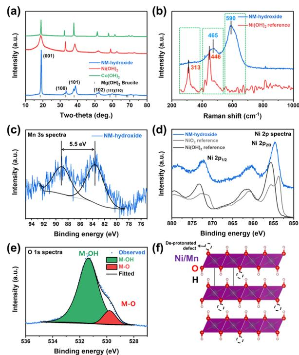
Fig. 1 Characterization of transition metal hydroxides: (a) XRD patterns of NM-hydroxide,  $\text{Ni}(\text{OH})_2$  reference and  $\text{Co}(\text{OH})_2$  reference and (b) Raman spectra of NM-hydroxide and  $\text{Ni}(\text{OH})_2$  reference. XPS spectra of NM-hydroxide: (c) Mn 3s, (d) Ni 2p and (e) O 1s core levels. (f) Crystal structure illustration of NM-hydroxide with de-protonated defects.
