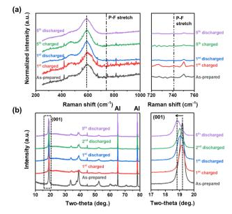
Fig. 4 (a) Raman spectra and (b) XRD patterns of the as-prepared, fully charged and fully discharged NM-hydroxide samples in different cycles.
