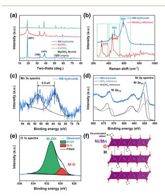
Fig. 1 Characterization of transition metal hydroxides: (a) XRD patterns of NM-hydroxide, Ni(OH)<sub>2</sub> reference and Co(OH)<sub>2</sub> reference and (b) Raman spectra of NM-hydroxide and Ni(OH)<sub>2</sub> reference. XPS spectra of NM-hydroxide: (c) Mn 3s, (d) Ni 2p and (e) O 1s core levels. (f) Crystal structure illustration of NM-hydroxide with de-protonated defects.
