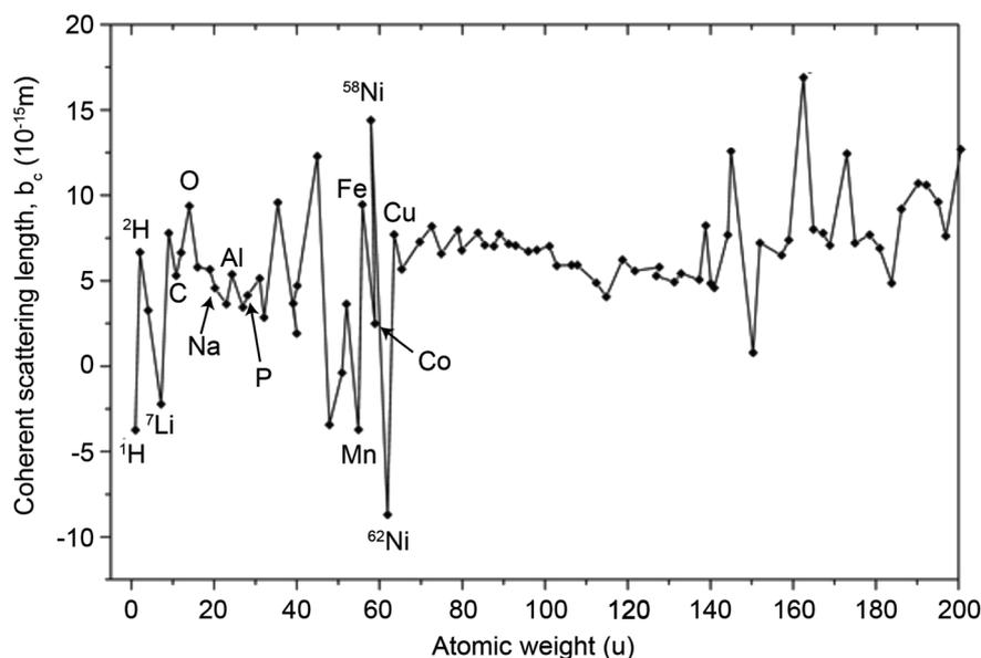
Fig. 6 Neutron scattering lengths of different isotopes (those relevant to battery materials are labelled). The magnitude of  $b$  is indicative of the isotope's scattering strength and its sign indicates a  $180^\circ$  phase difference relative to values with the opposite sign.
