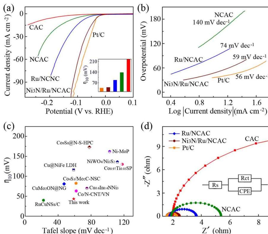
Fig. 3 (a) LSV curves of CACs, NCACs, Ru/NCACs,  $\text{Ni}_3\text{N}/\text{Ru}/\text{NCAC}$  composites and Pt/C catalysts (scan rate: 5  $\text{mV s}^{-1}$ ). Inset:  $\eta_{10}$  for these samples. (b) Tafel plots of samples in (a). (c) Comparison of  $\eta_{10}$  and the corresponding Tafel slopes with many reported high-performance HER electrocatalysts. The corresponding references are listed in Table S2.<sup>†</sup> (d) Nyquist plots of samples in (a).
