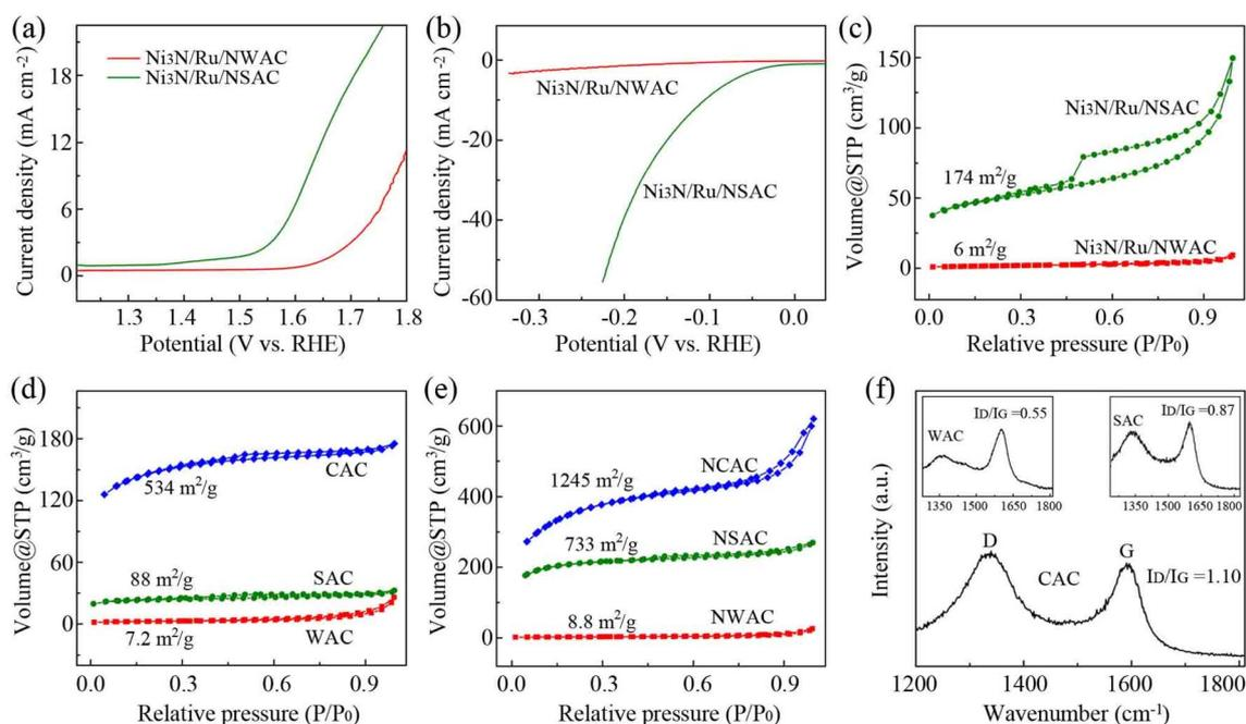
Fig. 4 (a, b) LSV curves of Ni<sub>3</sub>N/Ru/NWAC and Ni<sub>3</sub>N/Ru/NSAC composites for the OER and HER, respectively. Scan rate: 5 mV s<sup>-1</sup>. (c–e) Nitrogen adsorption–desorption isotherms. (c) Ni<sub>3</sub>N/Ru/NWAC and Ni<sub>3</sub>N/Ru/NSAC composites. (d) WACs, SACs and CACs. (e) NWACs, NSACs and NCACs. (f) Raman spectra of WACs, SACs and CACs.
