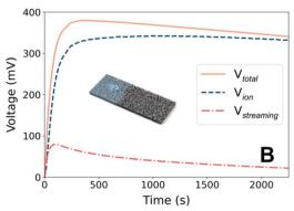
Fig. 2 (A). Comparison of the experimental voltage profile (black dots) and the model prediction (orange line). In the experiment, a 0.3 mL water droplet was placed on the left side of the carbon black-coated cotton fabric (inset). (B.) Voltage (defined as the potential difference between the head and tail ends of the substrate) predicted from the model (orange) and its decomposition into contributions from ions (navy) and streaming (red).
