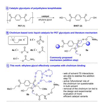
Fig. 1 Catalytic glycolysis of PET.
