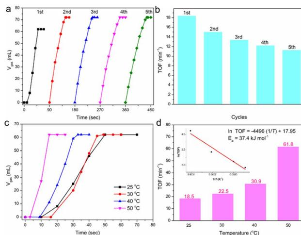
Fig. 1 (a and b) Durability of catalytic AB hydrolysis over 5 cycles at  $25^\circ\text{C}$ , and (c and d) temperature dependence of gas evolution of AB hydrolysis and the corresponding TOF values over Cu-Co-MOF-74 (inset in (d) is the Arrhenius plot ( $\ln \text{TOF}$ ) vs.  $1/T$ ) ( $n_{\text{Co}} = 0.204 \text{ mmol}$ ,  $n_{\text{Cu}} = 0.005 \text{ mmol}$ ,  $n_{\text{AB}} = 1 \text{ mmol}$ ).
