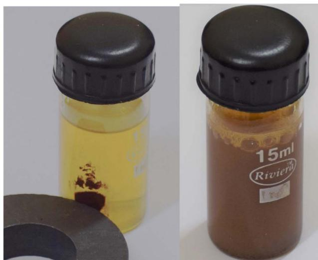
Fig. 11 Regeneration cycles of Co-Al31@Fe<sub>3</sub>O<sub>4</sub> and magnetic separation of the catalyst.
