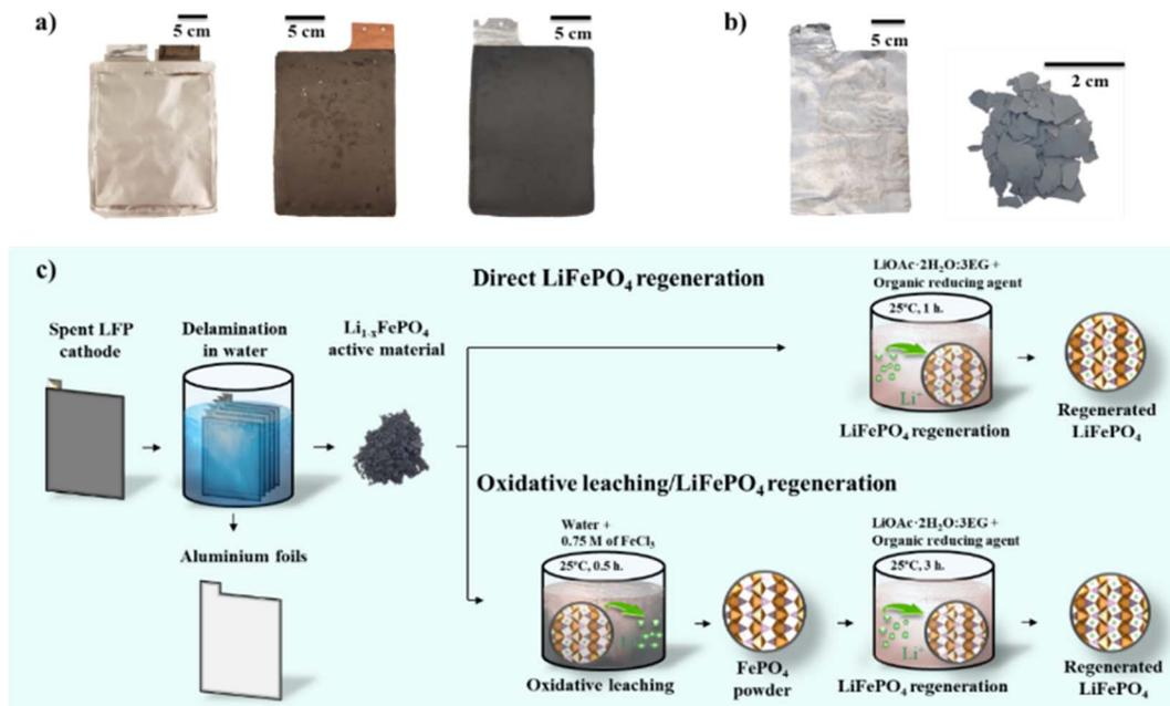
**Fig. 1** (a) Dismantled end-of-life pouch cell: a pouch case (left) anode plate (middle), and cathode plate (right), and (b) the materials generated after the delamination in water: delaminated aluminium foil (left) and cathode active material (right), and (c) schematic diagram showing the regeneration of  $\text{LiFePO}_4$  from spent  $\text{Li}_{1-x}\text{FePO}_4$  cathode.
