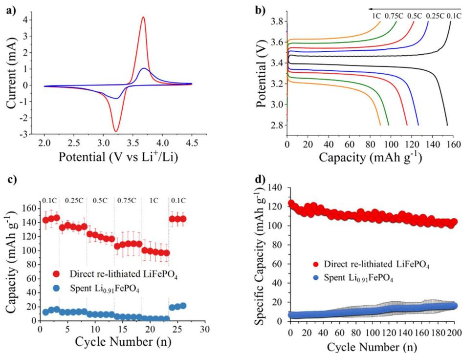
Fig. 5 (a) Cyclic voltammogram curves at a scan rate of  $0.2 \text{ mV s}^{-1}$  of direct re-lithiated  $\text{LiFePO}_4$  (b) the first charge and discharge curves of direct re-lithiated  $\text{LiFePO}_4$  at different discharge rates, (c) and (d) are rate capability, and cycle performance at 0.5C of direct re-lithiated  $\text{LiFePO}_4$  and spent  $\text{Li}_{0.91}\text{FePO}_4$ .
