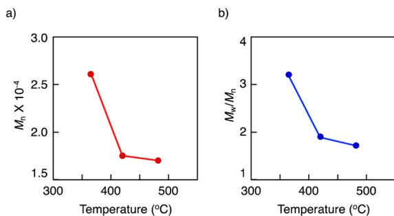
Fig. 13 Plots of (a) the molecular weight ( $M_n$ ) and (b) PDI ( $M_w/M_n$ ) of the residue versus temperature. Heating for 20 min.
