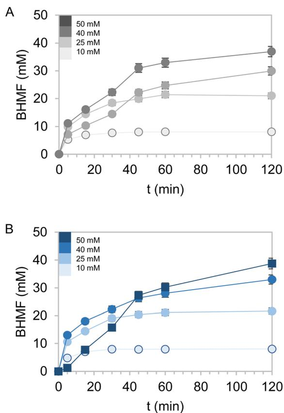
Fig. 5 HMF conversion by co-immobilised systems of EcADHZ3 and BsGDH-2M over Pu-E/Co<sup>2+</sup> (A) and Pu-G (B) at different substrate concentrations: 10 mM, 25 mM, 40 mM and 50 mM. Reaction mixtures contain equimolar amounts of glucose relative to HMF and 1 mM NADH in 100 mM Tris-HCl at pH 7.0 and 25 °C. Catalyst load  $0.1 \text{ g}_{\text{catalyst}} \text{ mL}^{-1}$ . In all cases, no by-products were detected, only the produced BHMF and the remaining HMF.
