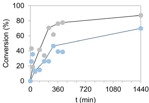
Fig. 7 HMF conversion by co-immobilised systems of EcADHZ3 and BsGDH-2M over Pu-E/Co<sup>2+</sup> (grey) and Pu-G (blue) with shifted w/v proportions (0.5 g in 125 mL). Reaction mixture contains 10 mM HMF, 25 mM glucose, NADH 1 mM, and 50 mM Tris-HCl buffer at pH 7.0, with a load of 0.004 g<sub>catalyst</sub> mL<sup>-1</sup>. The reaction is performed at 25 °C for 24 h.
