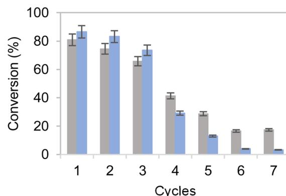
Fig. 6 Cycles of HMF conversion by co-immobilised systems of EcADHZ3 and BsGDH-2M over Pu-E/Co<sup>2+</sup> (grey) and Pu-G (blue). Reaction mixtures contain 40 mM HMF, 40 mM glucose, 1 mM NADH and 200 mM Tris-HCl buffer at pH 7.0, with a load of  $0.1 \text{ g}_{\text{catalyst}} \text{ mL}^{-1}$ . Each reaction cycle is performed at 25 °C for 24 h.
