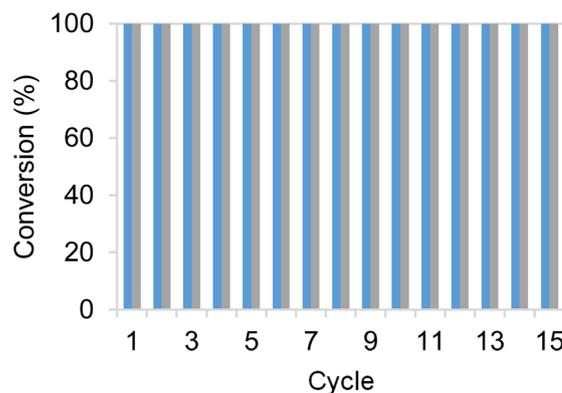
Fig. 4 Cycles of HMF conversion by co-immobilised systems of EcADHZ3 and BsGDH-2M on Pu-E/Co<sup>2+</sup> (grey) and Pu-G (blue). Reaction mixture contains HMF 10 mM, 25 mM glucose, and 1 mM NADH in 50 mM Tris-HCl buffer at pH 7.0, with a catalyst load of 0.1 g<sub>catalyst</sub> mL<sup>-1</sup>. Each reaction cycle is performed at 25 °C for 15 minutes.
