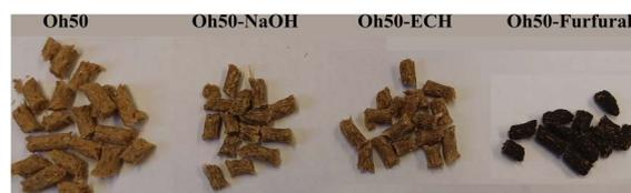
Fig. 1 Prepared composites from left to right: Oh50 (no NaOH), Oh50–NaOH, Oh50–ECH, and Oh50–Furfural.
