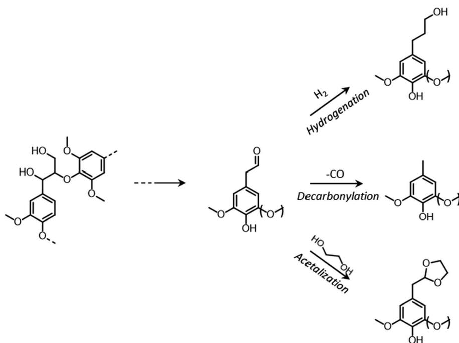
Fig. 26 Possible routes for the stabilization of C<sub>2</sub>-aldehyde-substituted phenolics during acid-catalyzed depolymerization of isolated lignin.
