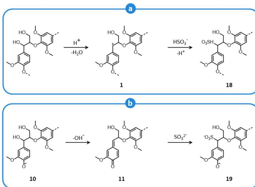
Fig. 12 Sulfonation of  $\beta\text{-O-4'}$  lignin motifs during sulfite pulping at acid conditions (a), and neutral/basic conditions (b). Based on Sjöström,<sup>150</sup> and Evtuguin.<sup>161</sup>
