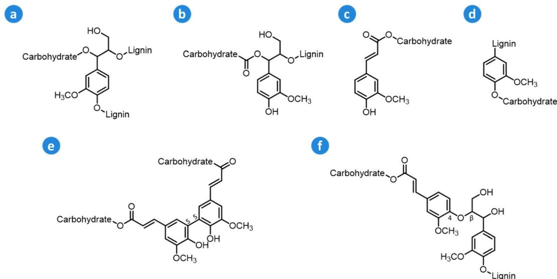
Fig. 6 Main types of LCC linkages: (a) benzyl ether, (b) benzyl ester, (c) ferulate ester, (d) phenyl glycosidic, (e) diferulate ester (5-5'), and (f) diferulate ester ( $\beta$ -O-4'). Based on Zhao *et al.*<sup>57</sup> and Tarasov *et al.*<sup>58</sup>
