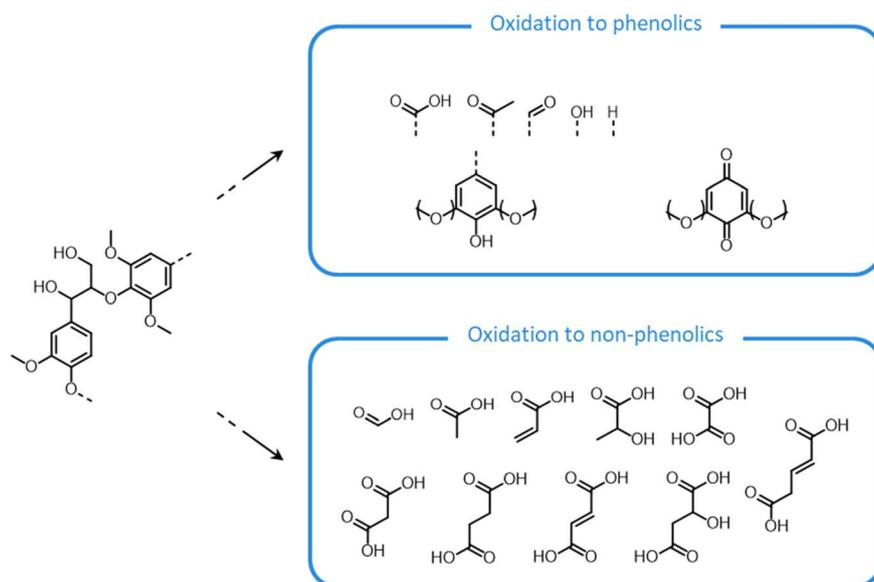
Fig. 24 Overview of phenolic monomers produced upon oxidative depolymerization of isolated lignin. Based on Schutyser *et al.*<sup>14</sup> Note: bonds other than β-O-4' linkages are cleaved during oxidative depolymerization, including both C–O and C–C bonds.
