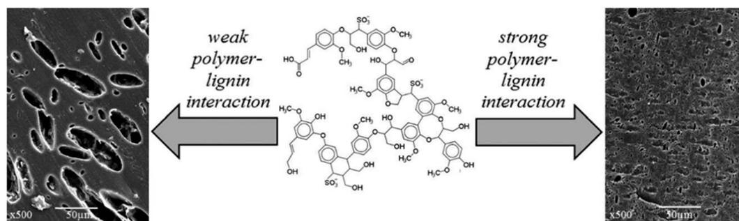
Fig. 21 Possible morphologies of lignin–polymer blends: heterogeneous blend with large dispersed particles (left) and homogeneous blend with no observable particles. Adapted from Kun *et al.*<sup>275</sup>
