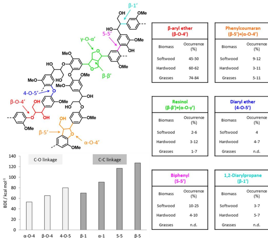
Fig. 5 Main lignin inter-unit linkage motifs with relative occurrence in different types of lignocellulose feedstocks and their bond dissociation energy (BDE). Based on Rinaldi *et al.*,<sup>15</sup> Wang and Wang,<sup>55</sup> and Parthasarathi *et al.*<sup>56</sup>
