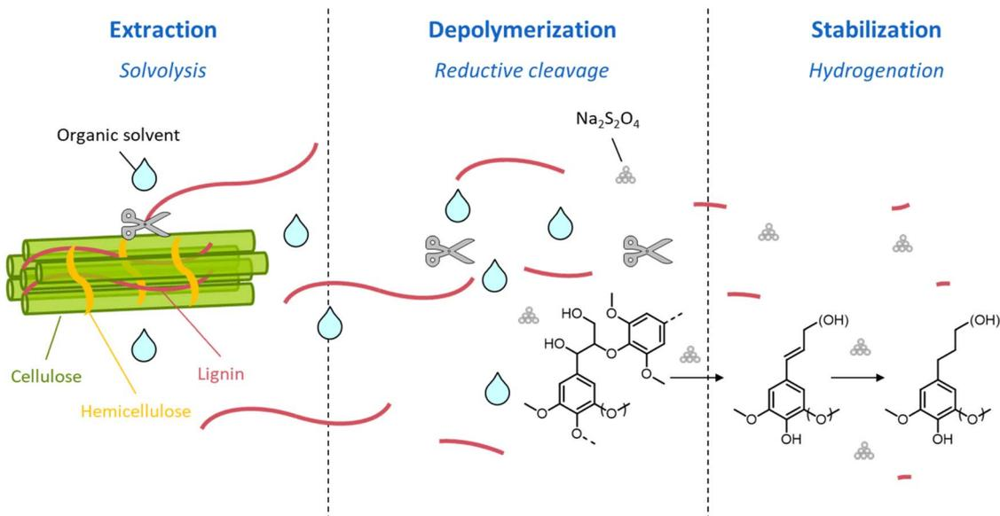
Fig. 44 Schematic representation of lignin extraction, depolymerization, and stabilization during DAOF. Based on Brienza *et al.*<sup>531</sup>
