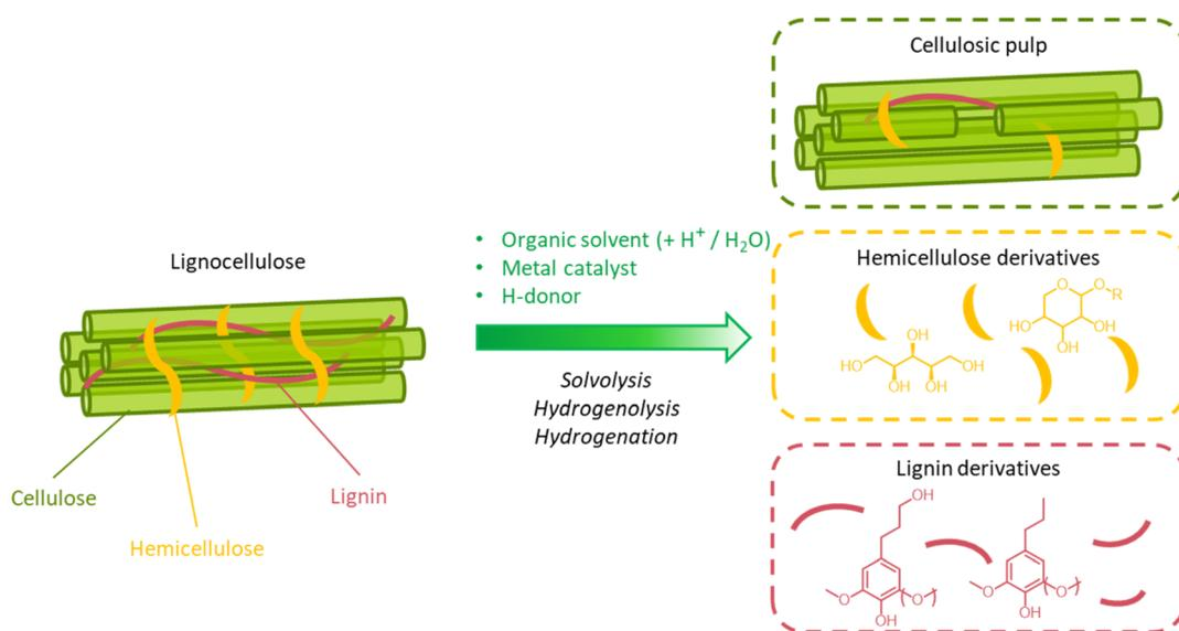
Fig. 37 Schematic outline of the RCF process for the extraction, depolymerization, and stabilization of lignin (and hemicellulose) derivatives from lignocellulosic biomass *via* solvolysis, solvolysis/hydrogenolysis, and hydrogenation, respectively. Note: when RCF is performed in the absence of water or without an acid co-catalyst, hemicellulose is mainly retained in the solid pulp.
