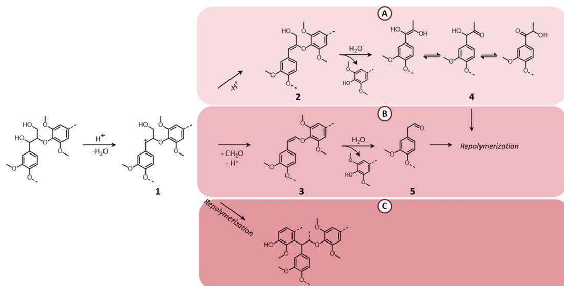
Fig. 7 Lignin chemistry in acidic conditions. Pathway A: formation of Hibbert's ketones; pathway B: formation of C<sub>2</sub>-aldehyde substituted phenolics; pathway C: repolymerization. Based on Liao *et al.*<sup>39</sup>
