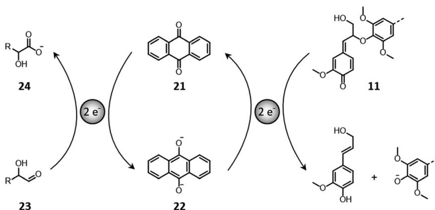
Fig. 14 Anthraquinone–anthrahydroquinone reactions with carbohydrates and lignin in alkaline conditions. Based on Sjöström.<sup>150</sup>
