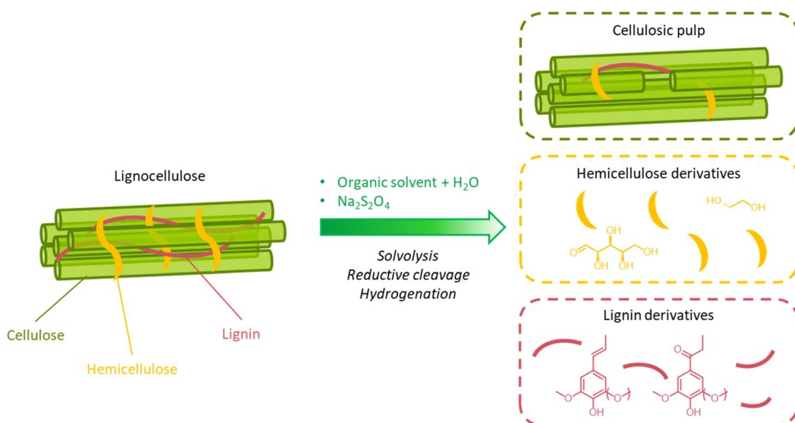
Fig. 45 Schematic outline of the DAOF process for the extraction, depolymerization, and stabilization of lignin derivatives from lignocellulosic biomass *via* reductive cleavage, and hydrogenation, respectively.
