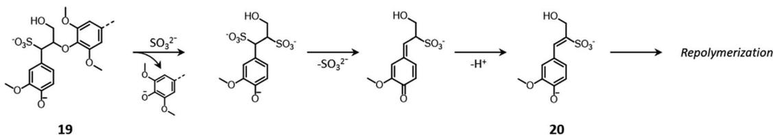
Fig. 13 Sulfitolysis of  $\beta$ -O-4' linkages during neutral/alkaline sulfite pulping. Based on Sjöström,<sup>150</sup> and Evtuguin.<sup>161</sup>
