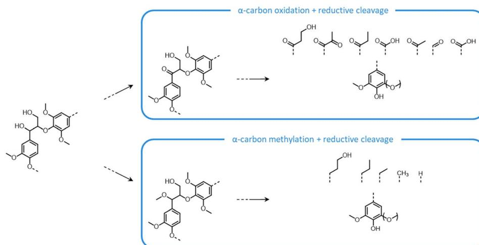
Fig. 23 Overview of phenolic monomers produced upon two-step reductive depolymerization of isolated lignin. Based on Schutyser *et al.*<sup>14</sup> and Sun *et al.*<sup>16</sup>
