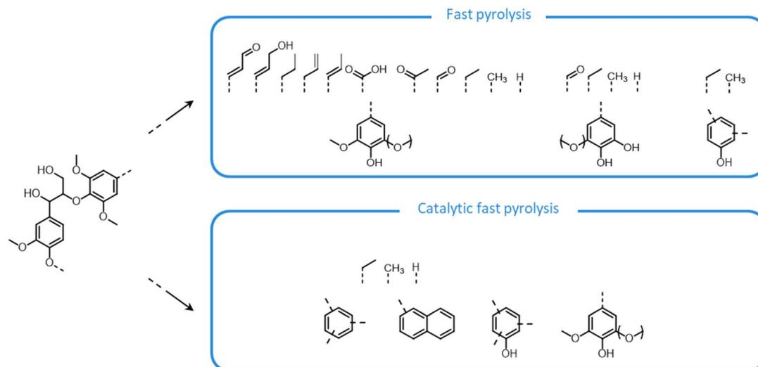
Fig. 29 Overview of phenolic monomers produced upon fast pyrolysis and catalytic fast pyrolysis of isolated lignin. Based on Schutyser *et al.*<sup>14</sup> Note: bonds other than  $\beta$ -O-4' linkages are cleaved during pyrolysis, including both C–O and C–C bonds.
