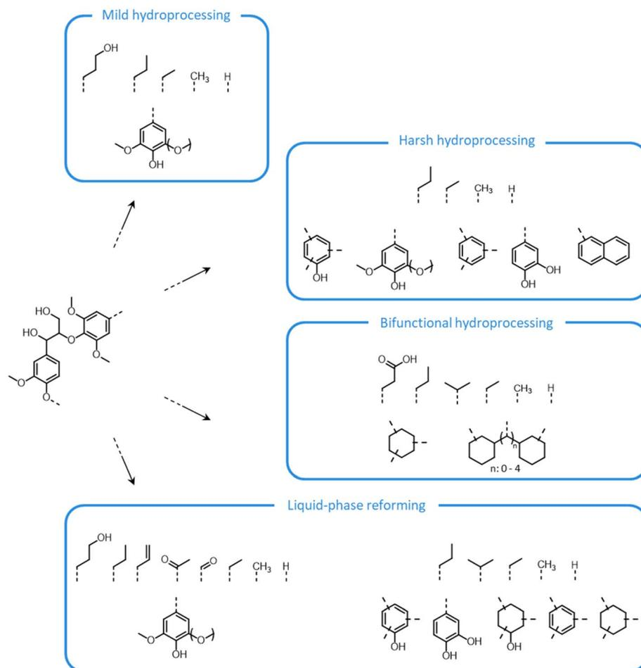
Fig. 22 Overview of phenolic monomers produced upon mild, harsh, and bifunctional hydroprocessing, and liquid-phase reforming of isolated lignin. Based on Schutyser *et al.*<sup>14</sup>
