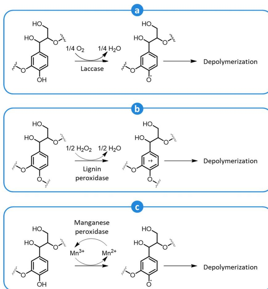
Fig. 18 Oxidative depolymerization of lignin by the action of laccase (a), lignin peroxidase (b), and manganese peroxidase (c). Adapted from Vasco-Correa *et al.*<sup>257</sup>
