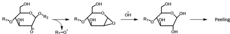
Fig. 11 Alkaline hydrolysis of carbohydrates in alkaline conditions. Based on Lachenal<sup>149</sup> and Gierer.<sup>157</sup>
