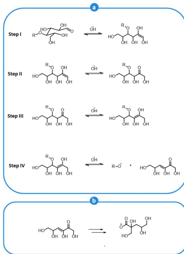
Fig. 10 Peeling reaction of carbohydrates in alkaline conditions (a), and fate of the eliminated units (b). Based on Lachenal<sup>149</sup> and Fearon *et al.*<sup>156</sup>
