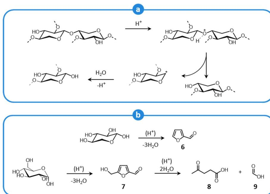
Fig. 8 Acid-catalyzed cleavage of glycosidic bonds (a) and possible decomposition reactions of the released sugar fragments (b). Based on Cybulska *et al.*,<sup>108</sup> and Xiao *et al.*<sup>109</sup>
