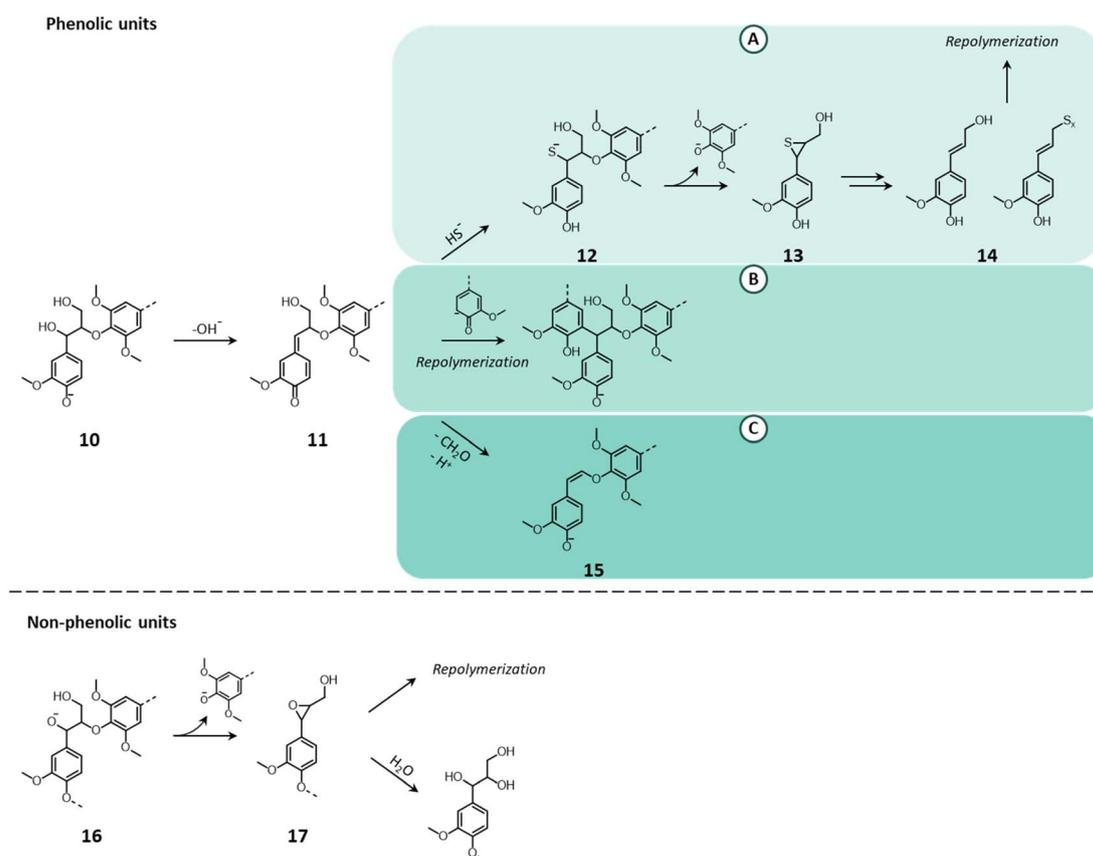
Fig. 9 Lignin chemistry in alkaline conditions. Pathway A: nucleophilic attack by HS<sup>-</sup>; pathway B: repolymerization; pathway C: loss of formaldehyde and enol ether formation. Based on Lachenal<sup>149</sup> and Rinaldi *et al.*<sup>15</sup>
