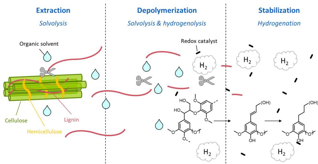
Fig. 36 Schematic representation of lignin extraction, depolymerization, and stabilization during the RCF. Based on Van den Bosch *et al.*<sup>460</sup>
