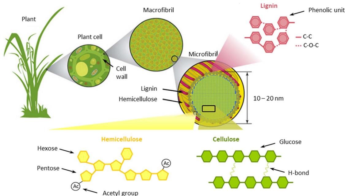
Fig. 1 Schematic structure of lignocellulose components. Modified from Potters *et al.*<sup>33</sup>
