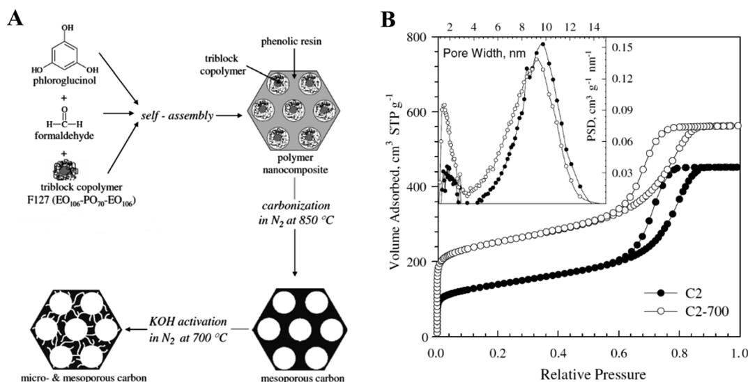
Fig. 3 (A) A common soft-templating system to prepare highly ordered mesoporous carbons, and then micropores on their wall via KOH activation. (B) N<sub>2</sub> adsorption–desorption isotherms before (C2) and after the KOH activation step (C2-700) (inset shows the pore size distribution derived from these isotherms). Reproduced from ref. 32 with slight modification. Copyright 2008 Elsevier.
