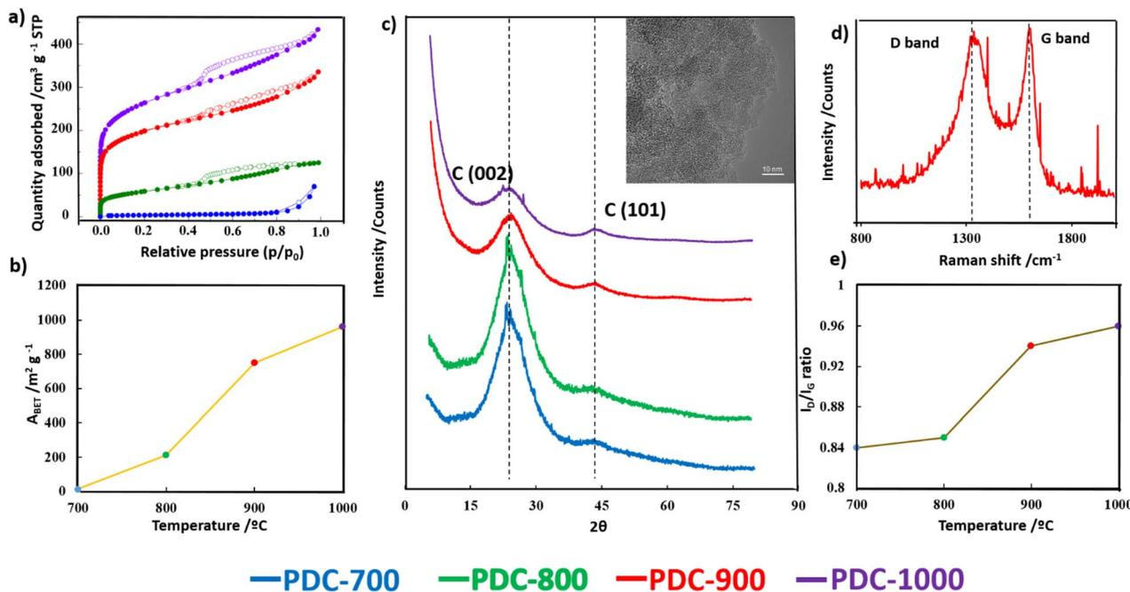
Fig. 2 (a) N<sub>2</sub> adsorption (full symbols) – desorption (empty symbols) isotherms of the PDC-*T* series; (b) plot of  $A_{\text{BET}}$  obtained from N<sub>2</sub> adsorption isotherms; (c) XRD patterns of the PDC-*T* series and TEM image of PDC-900 (inset); (d) Raman spectra of PDC-900; and (e) plot of  $I_{\text{D}}/I_{\text{G}}$  ratio obtained from Raman spectra.
