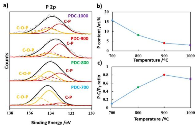
Fig. 3 (a) P 2p XPS spectra, (b) P content, and (c) P-C/P<sub>T</sub> ratio of the PDC-*T* series.
