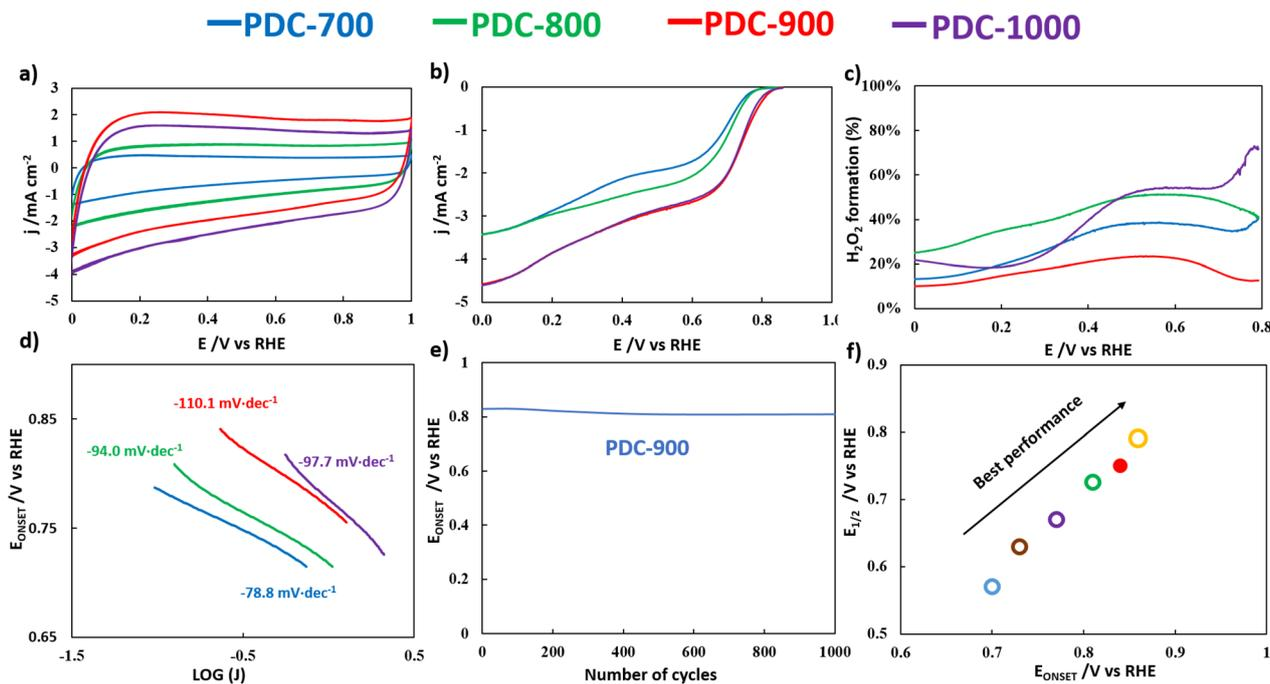
Fig. 4 (a) Cyclic voltammety in 0.1 M KOH, N<sub>2</sub>-saturated solution at 50 mV s<sup>-1</sup>; (b) linear sweep voltammety in 0.1 M KOH, O<sub>2</sub>-saturated solution at 1600 rpm; (c) H<sub>2</sub>O<sub>2</sub> formation; (d) Tafel slopes of all PDC-*T* materials; (e) stability of PDC-900 under continuous LSV cycling; (f) literature comparison of the ORR performance of other P-doped materials (unfilled circles) to PDC-900 (red solid circle).
