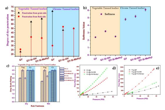
(a) Degree of dye penetration, (b) softness, (c) rub fastness and (d) and (e) air permeability of the chrome and vegetable-tanned leather.
