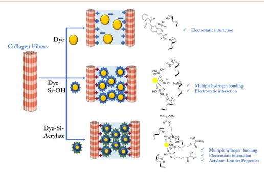
Scheme 2 Interactions between dye and collagen, dye-Si-OH and collagen, dye-Si-acrylate and collagen.
