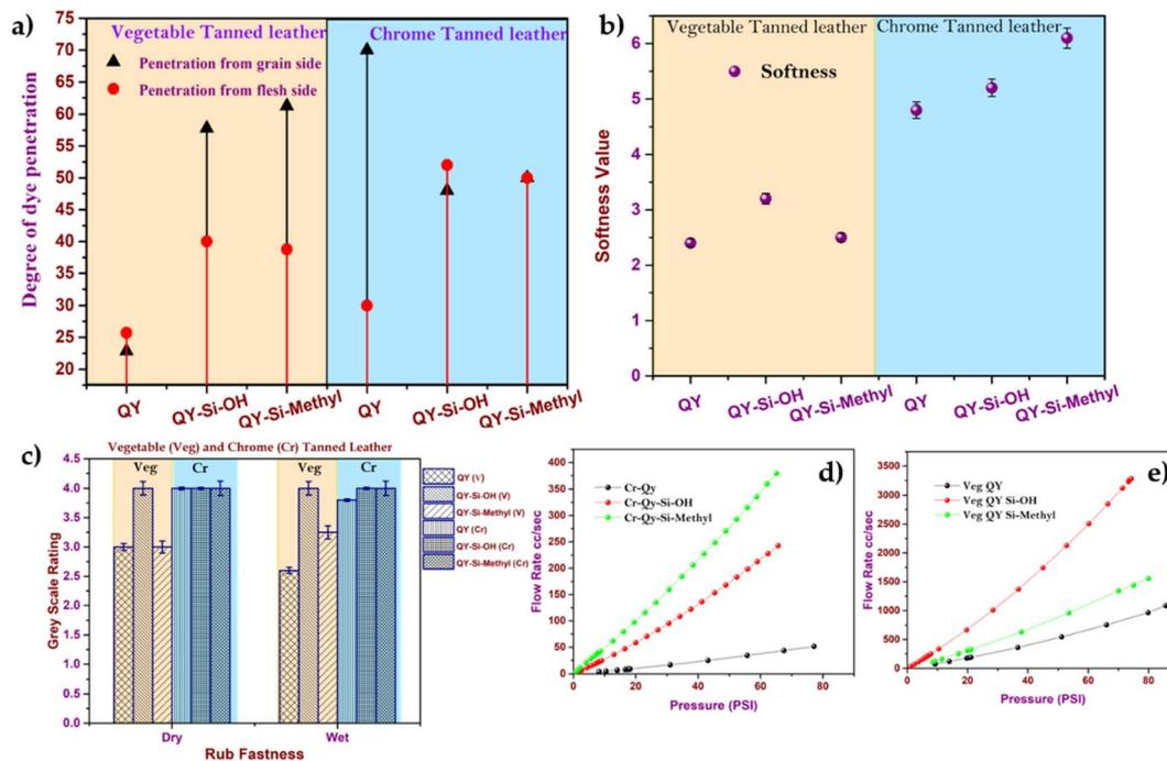
Fig. 5 (a) Degree of dye penetration, (b) softness, (c) rub fastness and (d) and (e) air permeability of the chrome and vegetable-tanned leather.
