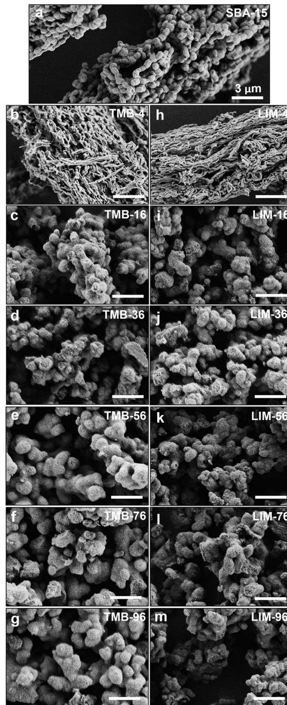
Fig. 5 SEM images of SBA-15 (a) and pore expanded micellar templated silica obtained with increasing amounts of expander TMB (left column) and limonene (right column). The scale bar is 3  $\mu$ m for all images.
