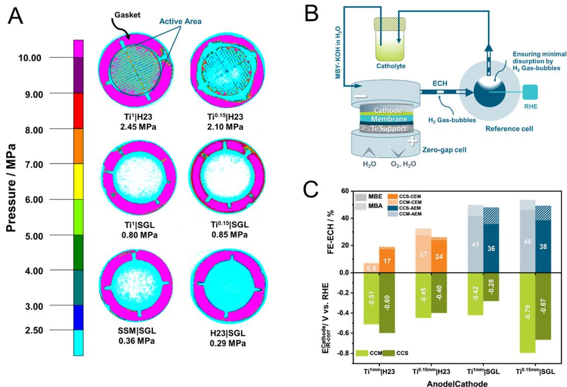
Fig. 2 Visualization of the applied pressure within the employed 12.57 cm<sup>2</sup> electrolyzer (A). Schematic representation of the modified set-up used to determine the half-cell voltages at the cathode (B). Investigation of the interplay between cathode half-cell potential and FE-ECH at 80 mA cm<sup>-2</sup> (catholyte: 1 MBY, 0.3 M KOH in H<sub>2</sub>O, anolyte: H<sub>2</sub>O) (C).
