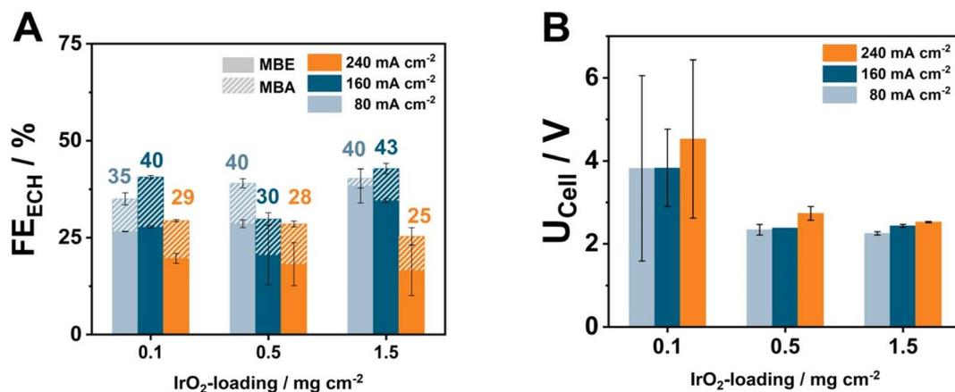
Fig. 4 Investigation of the effect of  $\text{IrO}_2$  loading on the CCM-AEM\_Ti<sup>0.15 mm</sup>|H<sub>23</sub> on the MBY-ECH at three different current densities (catholyte: 1 MBY, 0.3 M KOH in H<sub>2</sub>O, anolyte: 2 M KOH). Comparison of the obtained FE (A) and the respective cell voltages (B) after 1 h of electrolysis. Here the filled FE values denote the detected quantified FE for MBE, while the striped one represents the FE for MBA, detected in the catholyte.
