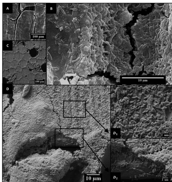
Fig. 3 SEM images of *G. sulfurreducens* biofilms grown on 1000 (A and C) and 600 °C biochar (B and D). Magnification of 1000 and 600 °C electrode micrographs (C and D1 and D2, respectively) clearly shows bacteria forming dense biofilms on both biochar electrodes. Nevertheless, the coverage of the surface is heterogeneous (D1 vs. D2).
