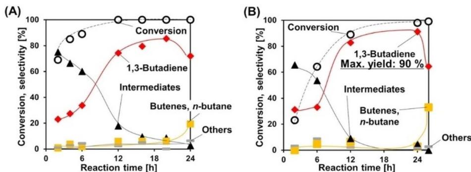
Fig. 1 Time courses in the deoxydehydration of erythritol over  $\text{ReO}_x\text{-Ag/CeO}_2$  (A) with 1,4-dioxane solvent and (B) without solvent. Reaction conditions:  $\text{ReO}_x\text{-Ag/CeO}_2$  (Re: 1 wt%, Ag/Re = 0.3 [mol mol<sup>-1</sup>]) 0.3 g, erythritol 0.25 g, 1,4-dioxane 4 g (A) or 0 g (B), 413 K,  $\text{H}_2$  8 MPa. Reprinted from ref. 115 with permission from Wiley-VCH.
