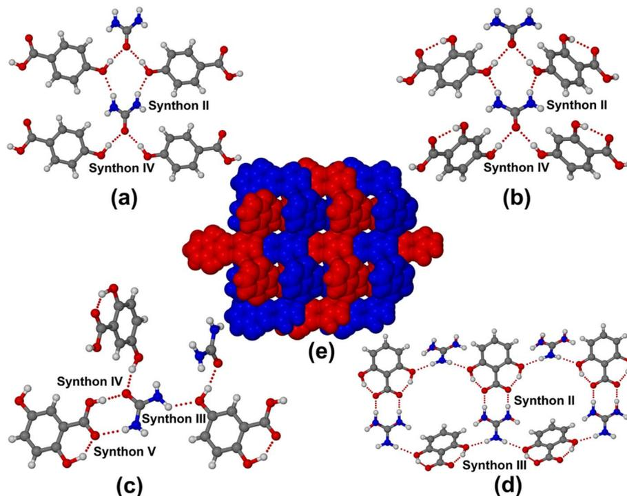
Fig. 1 Various hydrogen-bond synthons present in (a) urea·4HBA, (b) urea·24DHBA, (c) urea·25DHBA, and (d) urea·26DHBA and (e) 2-fold interpenetration of urea·26DHBA salt structure.
