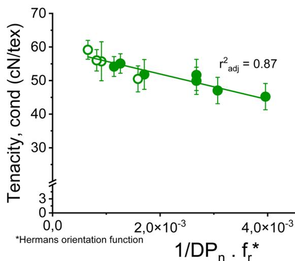
Fig. 13 Conditioned tenacity of Ioncell fibers with titers of  $1.21 \pm 0.10$  dtex made from SWS-IP (open circles) and HWPHK pulps (closed circles) as a function of the reciprocal  $DP_n$  times the Hermans orientation function  $f_r$ .
