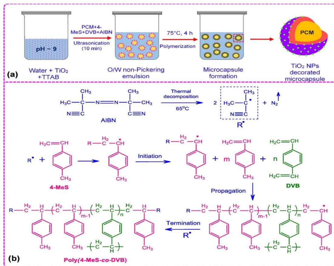
Fig. 7 (a) Schematic illustration for the creation of a crosslinked polystyrene-based shell decorated with TiO<sub>2</sub> nanoparticles and (b) free radical polymerization for the creation of the poly(4-methylstyrene-co-divinylbenzene) shell.<sup>47</sup> Reproduced with permission from ref. 47. Copyright 2021 ACS.
