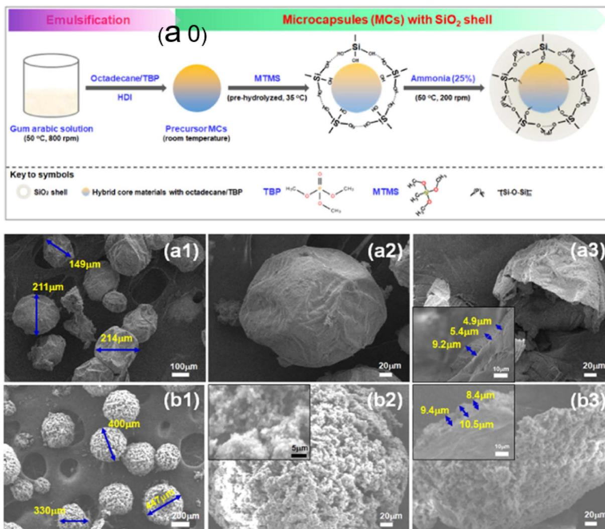
Fig. 13 (a0) Representation of microcapsule formation with a silica shell and an octadecane/TBP hybrid core, and SEM pictures of a hybrid MEPCM with  $\text{SiO}_2$  (a1–a3) and PUF (b1–b3).<sup>2</sup> Reproduced with permission from ref. 2 Copyright 2021 ACS.
