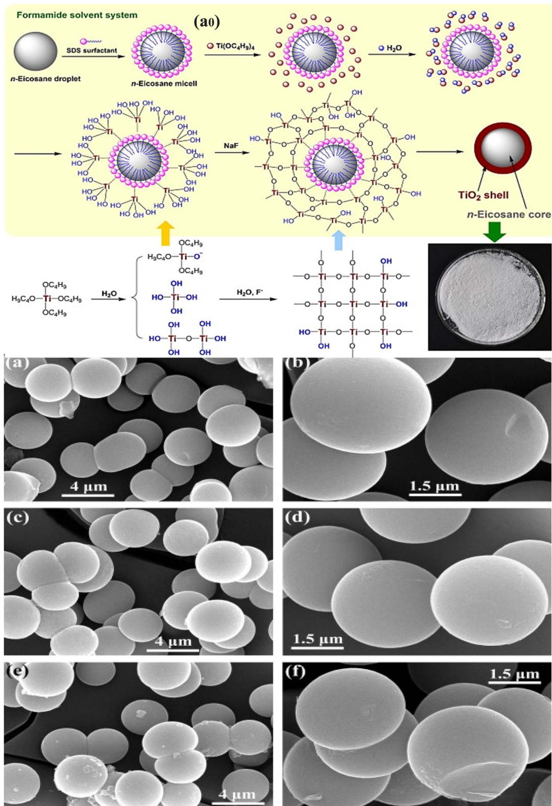
Fig. 15 (a0) Schematic illustration of the fabrication of the *n*-eicosane microcapsule  $\text{TiO}_2$  shell, SEM images of the *n*-eicosane microcapsule (a and b) produced with a weight ratio of 60/40 *n*-eicosane/TBT, (c and d) produced with a weight ratio of 50/50 *n*-eicosane/TBT, and (e and f) produced with a weight ratio of 40/60 *n*-eicosane/TBT.<sup>129</sup> Reproduced with permission from ref. 129 Copyright 2015 Elsevier.
