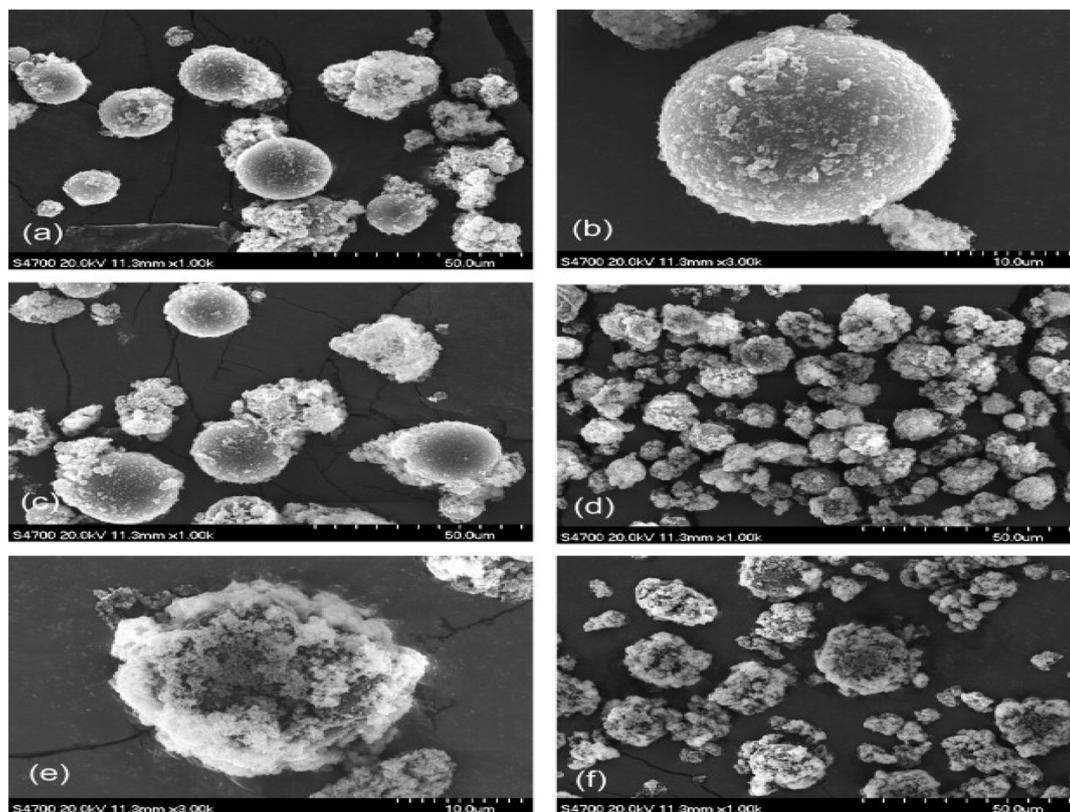
Fig. 2 (a0) Schematic illustration of the preparation of the MPCMs based on an octadecane core and modified MF-based shell, and SEM pictures of the microcapsules with various weight ratios of core/shell materials; (a) and (b) 65/35 (c) 75/25 using SMA as a surfactant, (d) and (e) 70/30 and (f) 75/25 using SDS as a surfactant.<sup>138</sup> Reproduced with permission from ref. 138. Copyright 2019 Elsevier.
