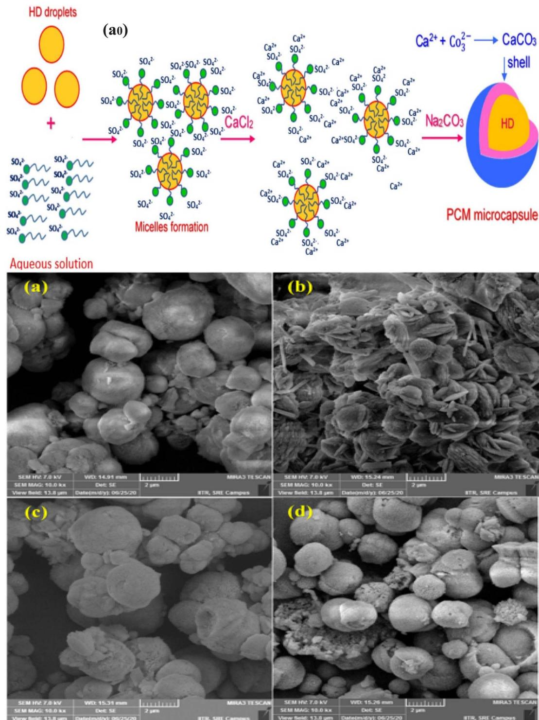
**Fig. 18** (a0) Schematic illustration of the preparation of hexadecane (core) with a calcium carbonate shell, (a–d) SEM pictures of MPCM capsules, (a) synthesized by using only SDS, (b) synthesized by using only PVP, (c) synthesized by using SDS and PVP surfactants at a 3 : 1 (SDS/PVP) weight ratio and (d) synthesized by using SDS and PVP surfactants at a 1 : 1 (SDS/PVP).<sup>174</sup> Reproduced with permission from ref. 174 Copyright 2022 Elsevier.
