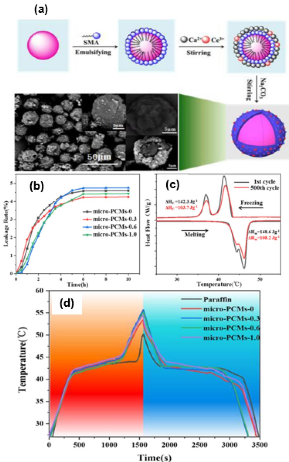
Fig. 19 (a) Schematic of synthesis for paraffin microcapsules composed of  $\text{Ce}^{3+}$  doped calcium carbonate with SEM images; (b) Leakage rate of paraffin microcapsules; (c) DSC curves of PCM microcapsules containing 0.6 wt%  $\text{Ce}^{3+}$  with respect to calcium carbonate; (d) paraffin and paraffin microcapsules' temperature–time curves during the release processes (blue) and storage (red).<sup>177</sup> Reproduced with permission from ref. 177 Copyright 2019 ACS.
