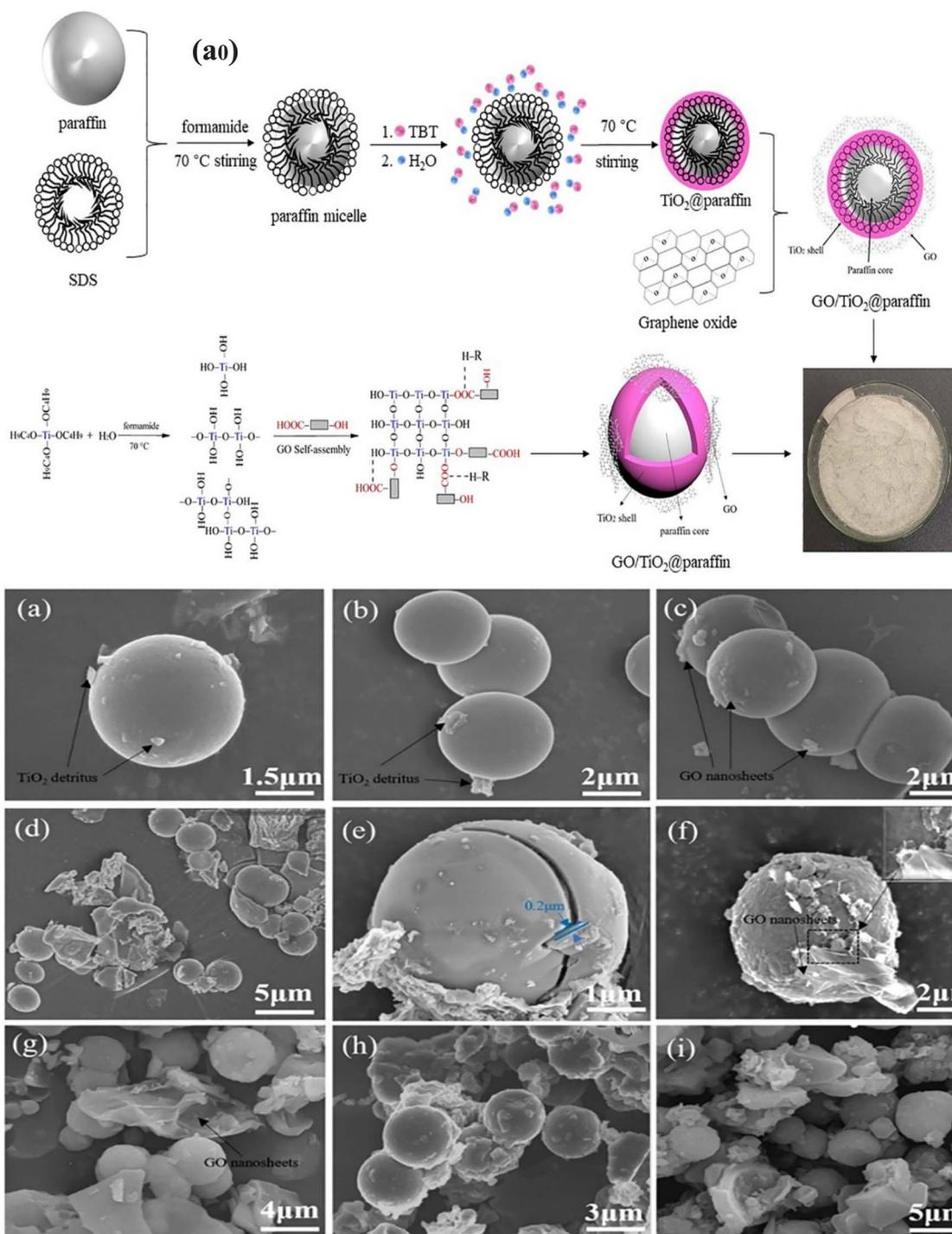
Fig. 14 (a0) Schematic illustration of the method for creating GO/TiO<sub>2</sub>/paraffin microcapsules, SEM images of (a and b) TiO<sub>2</sub>/paraffin microcapsules, (c and d) GO/TiO<sub>2</sub>/paraffin microcapsules containing 1 wt% GO, (e–g) GO/TiO<sub>2</sub>/paraffin microcapsules containing 2 wt% GO, and (h and i) GO/TiO<sub>2</sub>/paraffin microcapsules containing 3 wt% GO.<sup>163</sup> Reproduced with permission from ref. 163 Copyright 2021 Elsevier.
