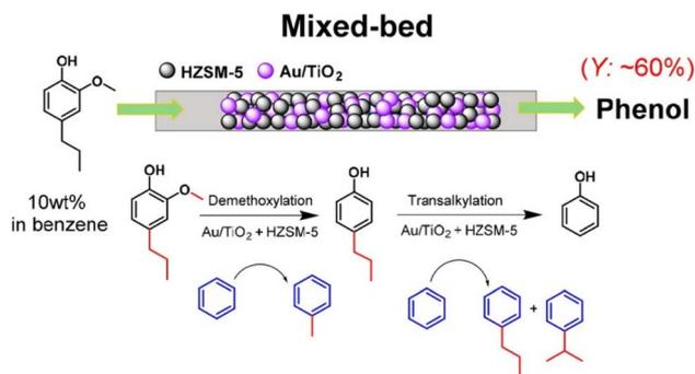
Fig. 3 One step process for demethoxylation and dealkylation over a mixed bed of Au/TiO<sub>2</sub> and HZSM-5 catalysts in benzene using a fixed-bed reactor. Reprinted from (ref. 87).
