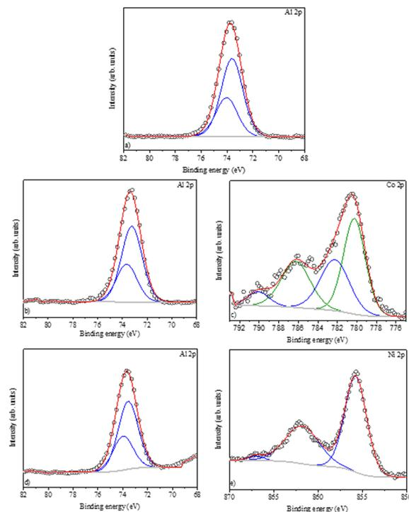
Fig. 7 XPS spectra: (a) Al2p –  $\text{Al}_2\text{O}_3$  (alumina), (b) Al2p –  $\text{CoAl}_2\text{O}_4$  (cobalt aluminate), (c) Co2p –  $\text{CoAl}_2\text{O}_4$  (cobalt aluminate), (d) Al2p –  $\text{NiAl}_2\text{O}_4$  (nickel aluminate), and (e) Ni2p –  $\text{NiAl}_2\text{O}_4$  (nickel aluminate).
