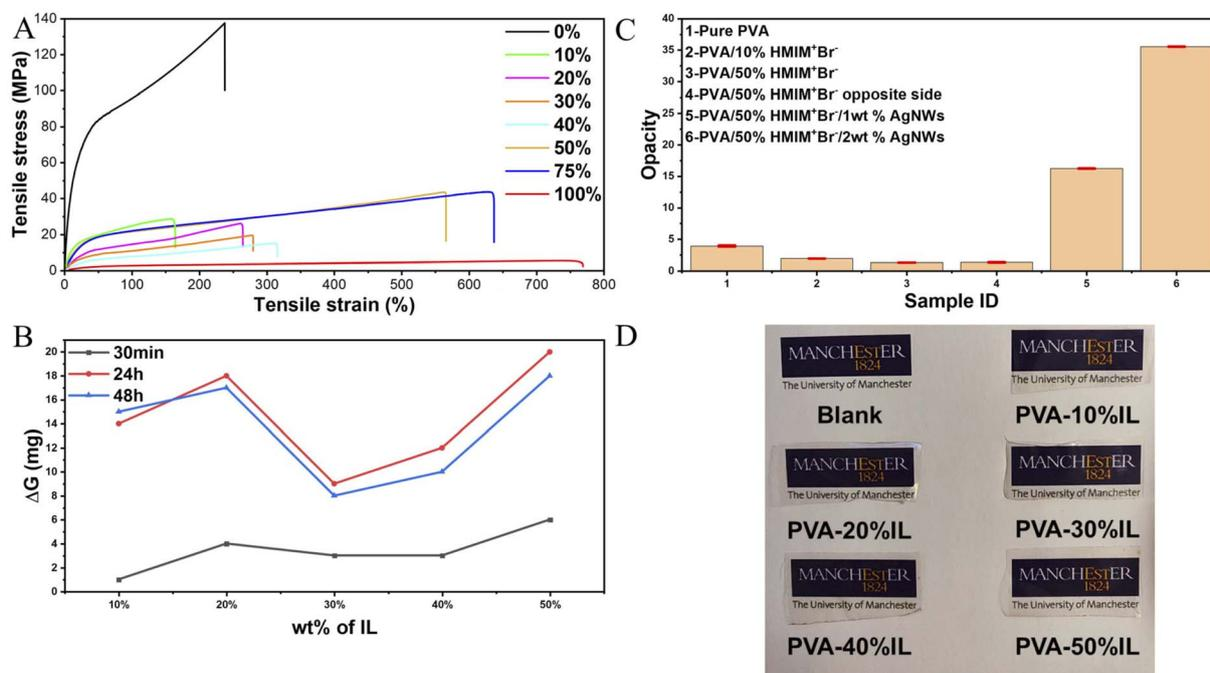
Fig. 3 (A) Tensile stress–strain curves, (B) moisture regain, (C) opacity, and (D) photographs of PVA films with different concentrations of [HMIM]<sup>+</sup>Br<sup>-</sup>.
