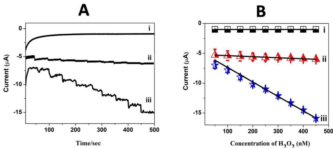
Fig. 8 (A) Chronoamperometric curves for the successive addition of  $\text{H}_2\text{O}_2$  (10 to 100 nM) in pH 7 PBS at (i) the bare GCE, (ii) GCE/poly(CoTBImPc) and (iii) GCE/CNT/poly(CoTBImPc) at  $-0.45 \text{ V}$  under stirring condition. (B) Plot of amperometric current vs. conc. of  $\text{H}_2\text{O}_2$  on different electrodes.
