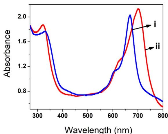
Fig. 11 Absorption spectra for (i) poly(CoTBImPc) and (ii) poly(CoTBImPc) and  $\text{H}_2\text{O}_2$  in DMSO solvent.
