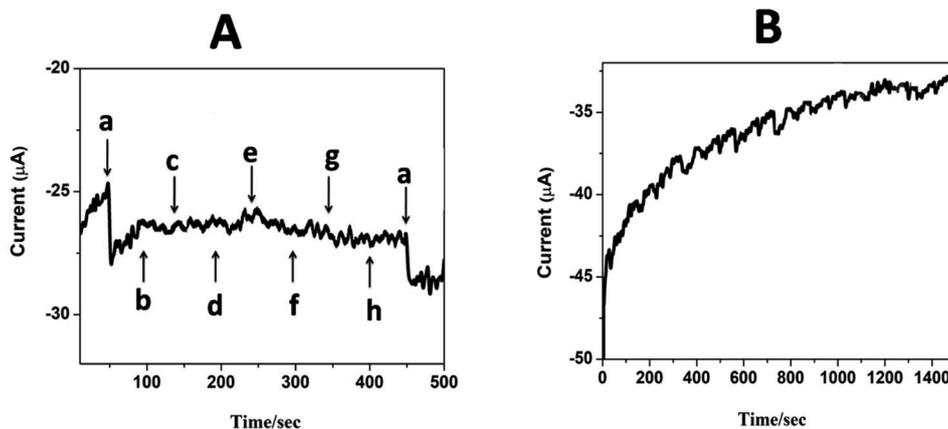
Fig. 9 (A) Amperometric  $i-t$  response for (a) 20 nM  $\text{H}_2\text{O}_2$  and 1 mM (b) glucose, (c) ascorbic acid, (d) dopamine, (e)  $\text{NaNO}_2$ , (f) hydroquinone, (g) KCl and (h)  $\text{KNO}_3$  in pH 7 PBS at GCE/CNP-poly(CoTBImPc).
