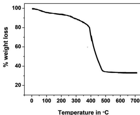
Fig. 3 TGA analytical curve for polyCoTBlmPc.
