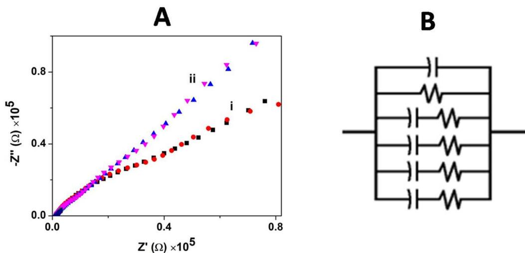
Fig. 6 (A) Impedance spectra for (i) the bare GCE and (ii) GCE/CNT/poly(CoTBImPc) in 0.1 mM  $[\text{Fe}(\text{CN})_6]^{3-/4-}$  in PBS. (B) Equivalent circuit used to fit the Nyquist plot.
