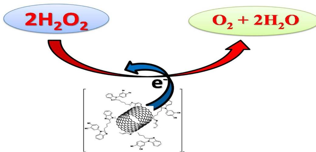
Fig. 10 Mechanism of  $\text{H}_2\text{O}_2$  reduction at the CNT/poly(CoTBImPc) electrode.
