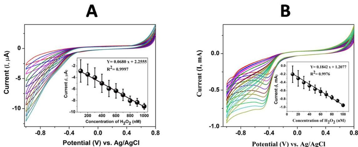
Fig. 7 Cyclic voltammograms at (A) GCE/poly(CoTBImPc) for different concentrations of  $\text{H}_2\text{O}_2$  (100 to 1000 nM) and (B) GCE/CNT/poly(CoTBImPc) for different concentrations of  $\text{H}_2\text{O}_2$  (10 to 100 nM) in PBS. Inset: plot of anodic peak current vs.  $\text{H}_2\text{O}_2$  concentration at  $-0.45$  V.
