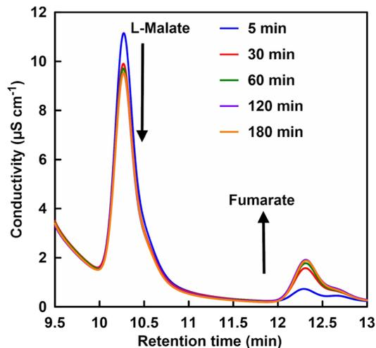
Fig. 4 A chart of an ion chromatogram sampled from the reaction solution containing L-malate, FUM and phosphate in HEPES buffer (pH 7.0).
