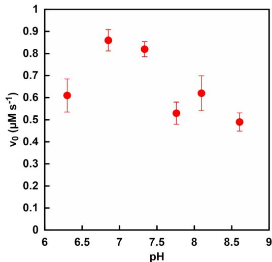
Fig. 2 The pH dependence on the initial rate of fumarate production ( $v_0$ ) with the system of sodium L-malate and FUM in HEPES buffer with varying pH from 6.3 to 8.6. Each plot shows the mean error of multiple measurements.
