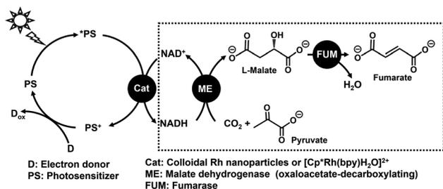
Fig. 1 Visible-light driven fumarate production from pyruvate and CO<sub>2</sub> with the system of an electron donor (D), a photosensitizer (PS), a catalyst for NADH regeneration, ME and FUM.
