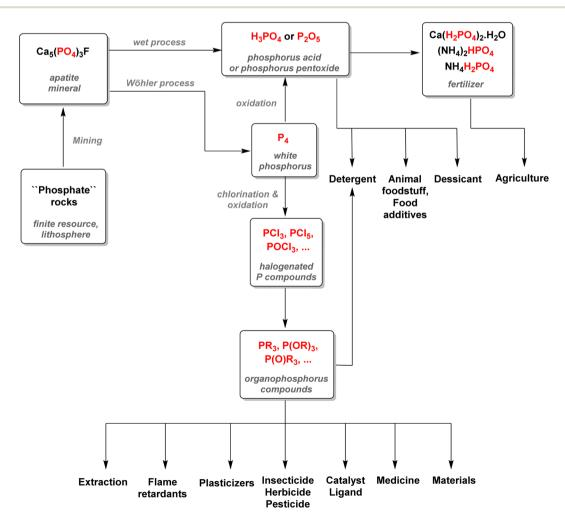
Fig. 4 Overview of the phosphorus industry and application.
