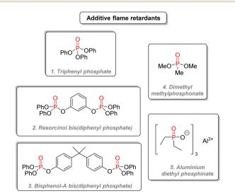
Fig. 30 P(v) organophosphorus as additive flame retardants.
