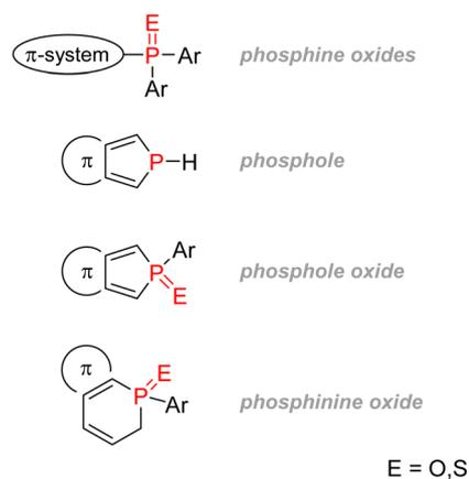
Fig. 23 Common organophosphorus structures for organic electronics.
