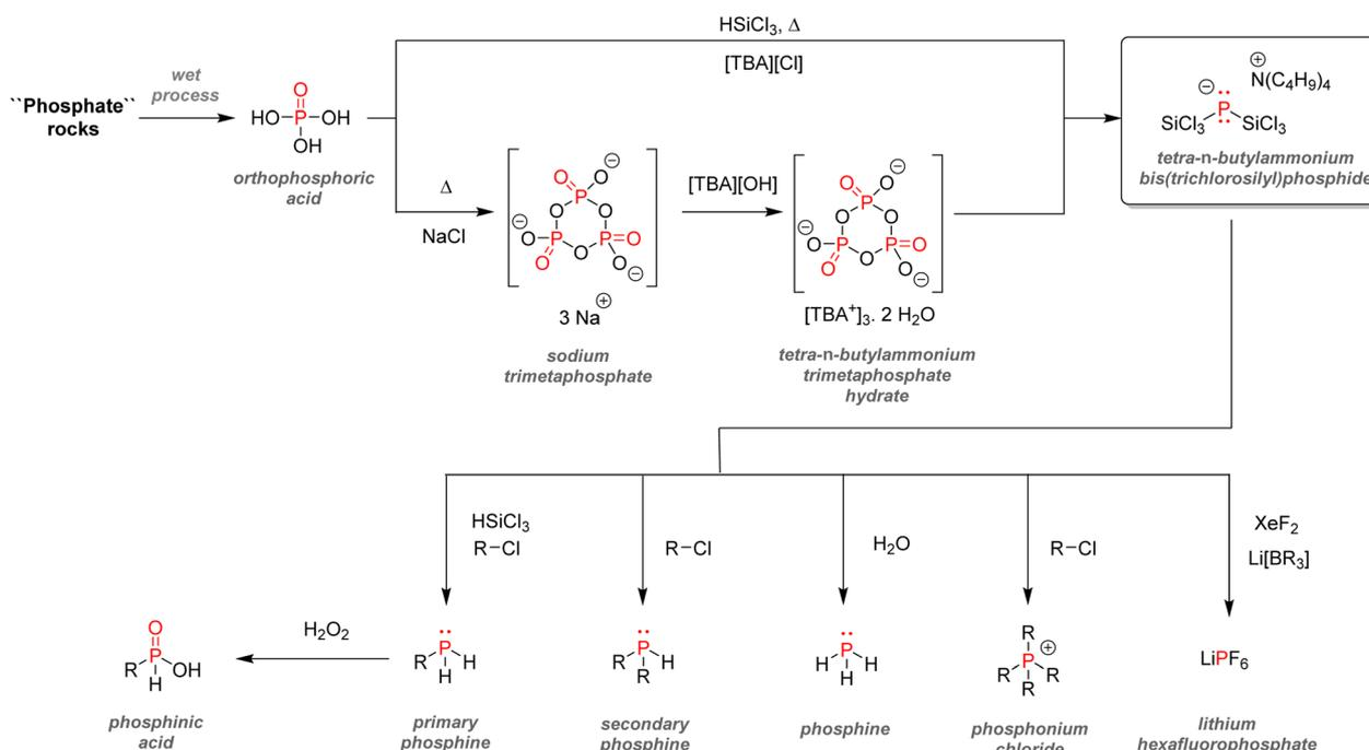
Fig. 37 Bis(trichlorosilyl)phosphide salts as intermediates for organophosphorus synthesis.
