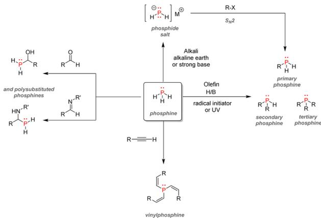
Fig. 36 Phosphine as an intermediate for organophosphorus synthesis.
